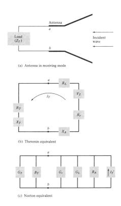
The power delivered to the load impedance is given by:
