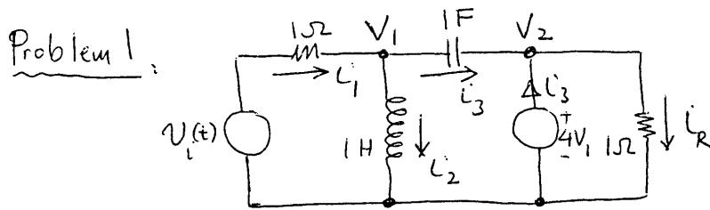
Write the differential equation for each energy storage element.
