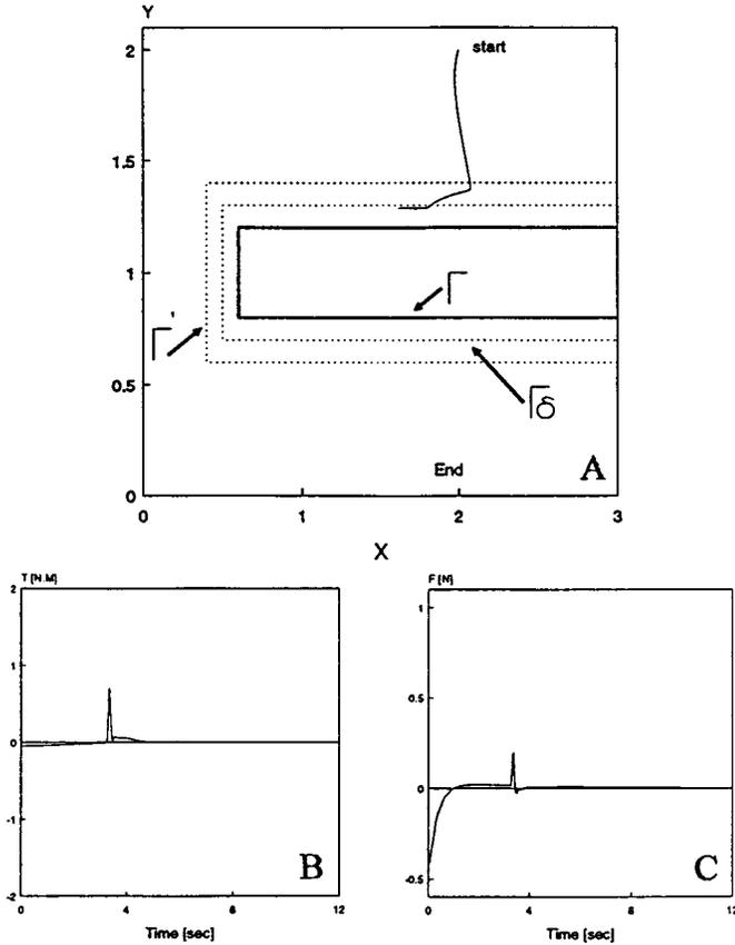
Fig. 15. Obstacle present, PPC, clamping, and nonlinear anisotropic damping controls used: (a) trajectory, (b) torque, and (c) force.
