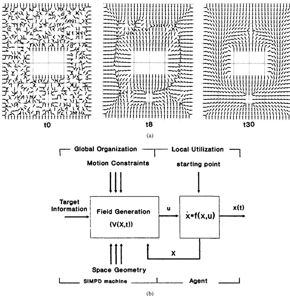
Fig. 2. (a) Evolution of a valid control group structure in a NC constructed using a hybrid, PDE-ODE, potential-based system. (b) Basic structure of a hybrid, PDE-ODE, Potential-based planning method.
