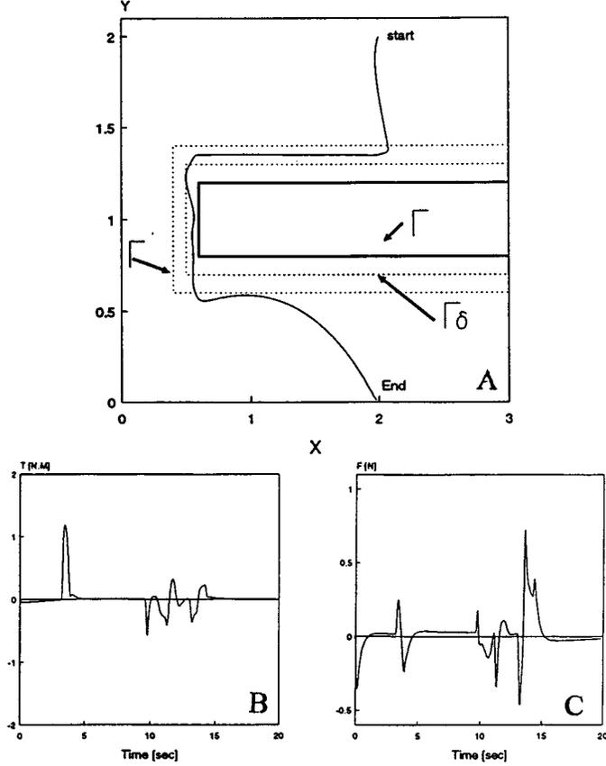
Fig. 16. Obstacle present, PPC, LAC, clamping, nonlinear anisotropic damping controls used: (a) trajectory, (b) torque, and (c) force.
