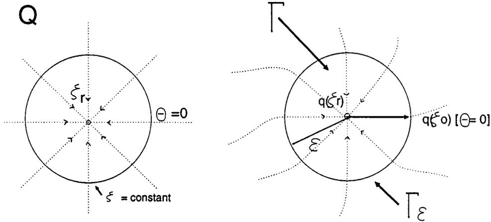
Fig. 20. Field lines near the exit point on the surface of the obstacle ( $\Gamma$ ) and its image  $Q$ .
