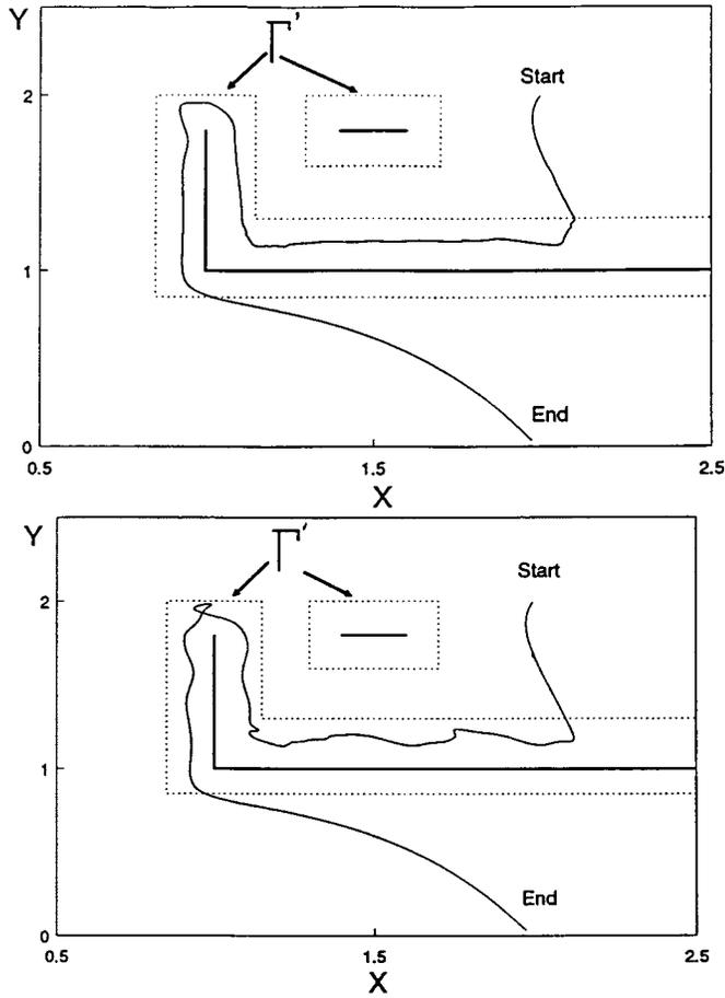
Fig. 19. (a) Robot trajectory, nonconvex obstacle, PPC, LAC, clamping, and damping controls present. (b) Removal of the damping control results in a shaky trajectory.
