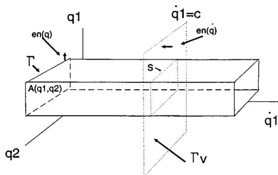
Fig. 4. Hyper-cylinders representing the velocity and position avoidance regions and their intersection  $S$ .
