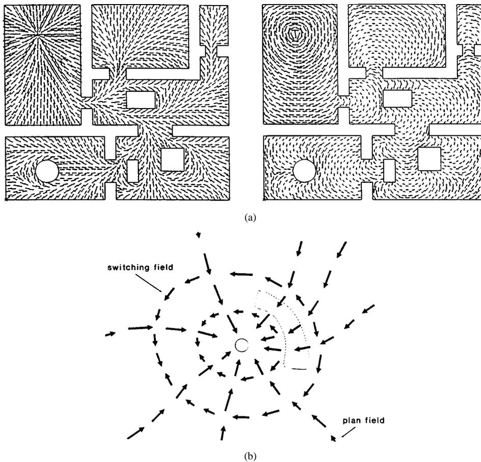
Fig. 3. (a) A general, curvilinear, boundary-fitted coordinate system from a vector potential realized by two gradient fields from scalar potentials. (b) Switching field from a VPF augmenting a plan field from a SPF.
