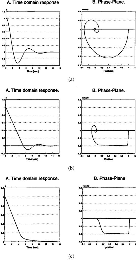
Fig. 10 (a) Unconstrained system,  $\zeta$ . (b) Velocity constrained not to go below  $-0.2$ . (c) Velocity constrained not to go below  $-0.2$ , and position constrained not to go below  $0.0$ .
