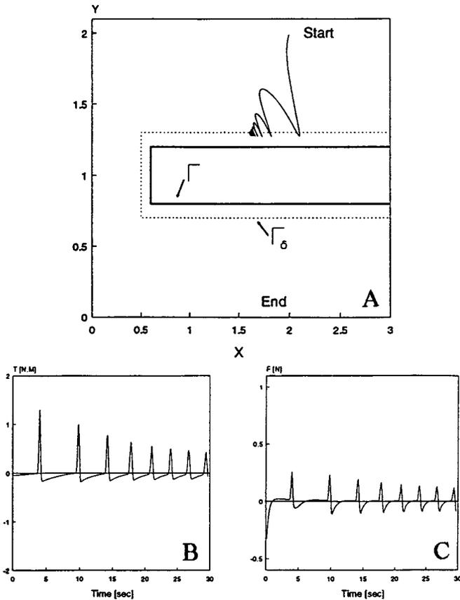
Fig. 13. Obstacle present, only PPC is used, (a) trajectory, (b) torque, (c) force.
