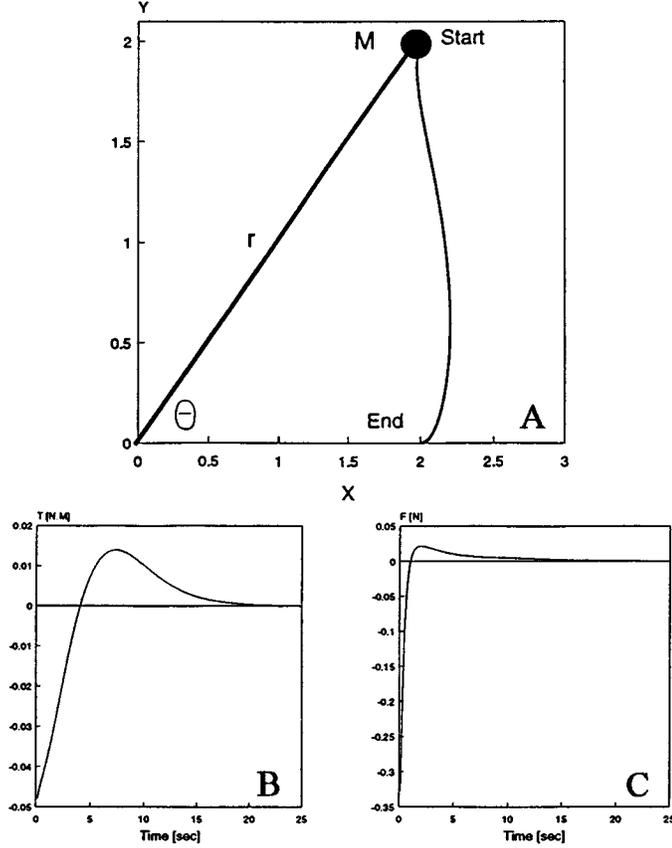
Fig. 12. (a) Robot trajectory in free space, (b) corresponding torque, and (c) corresponding force.
