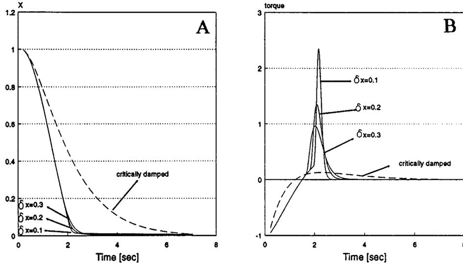
Fig. 11. (a) Response to different values of  $\delta_x$ , (b). corresponding forces.
