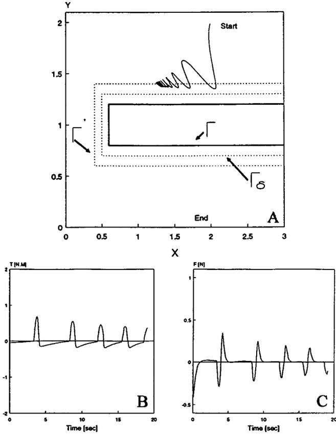
Fig. 18. Both damping and clamping controls removed, (a) trajectory, (b) torque, and (c) force.
