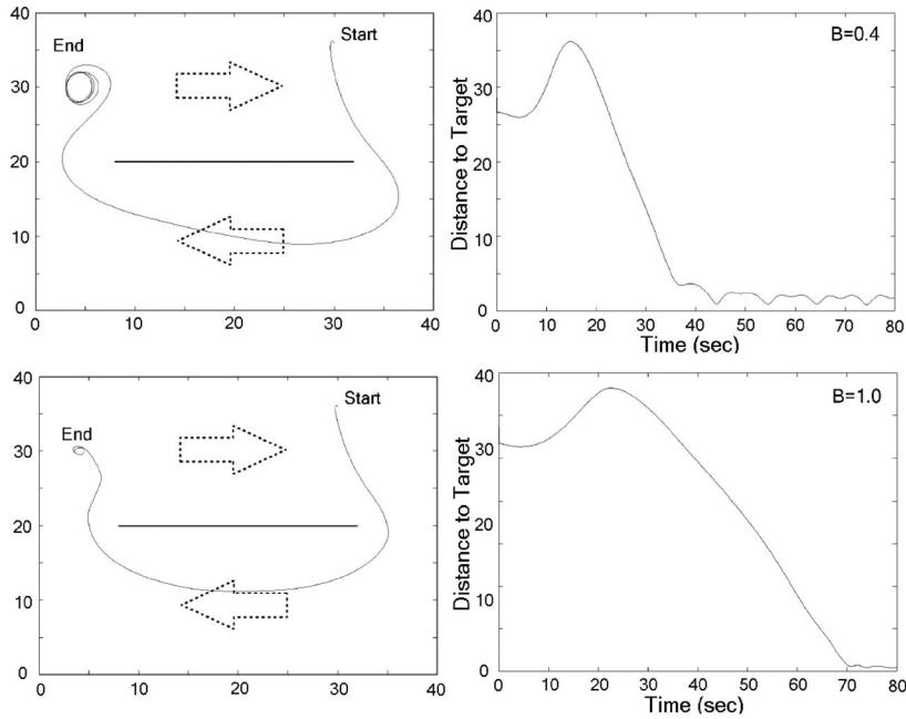
Fig. 3. Increasing  $B$  reduces transients but slows down motion.
