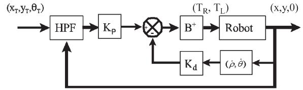
Fig. 14. Dynamic HPF-based planner with linear damping; nonholonomic case.
