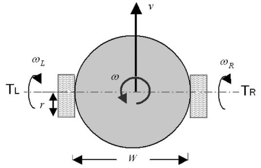
Fig. 9. Differential drive mobile robot.
