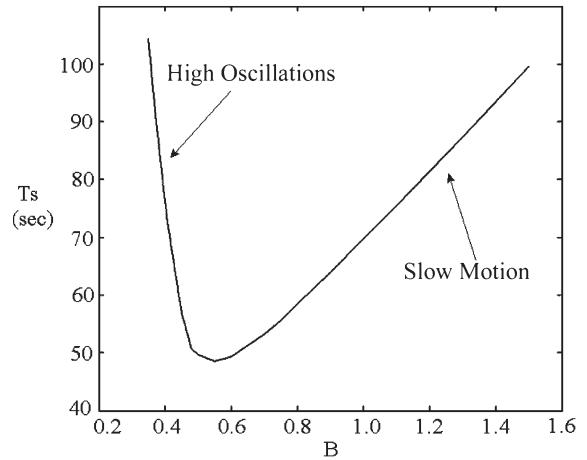
Fig. 7.  $T_S$  versus  $B$  for linear damping.
