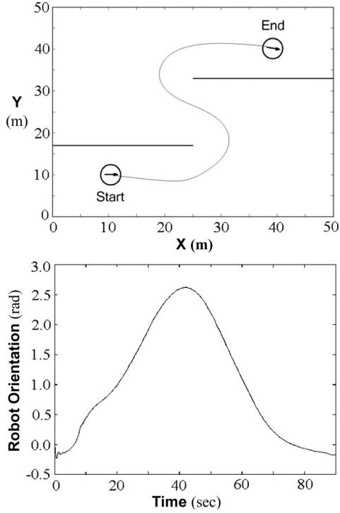
Fig. 19. Trajectory and curvature using the planner in (16) and the guidance field in Fig. 18.
