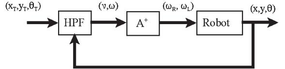
Fig. 10. Kinematic HPF-based planner; nonholonomic case.
