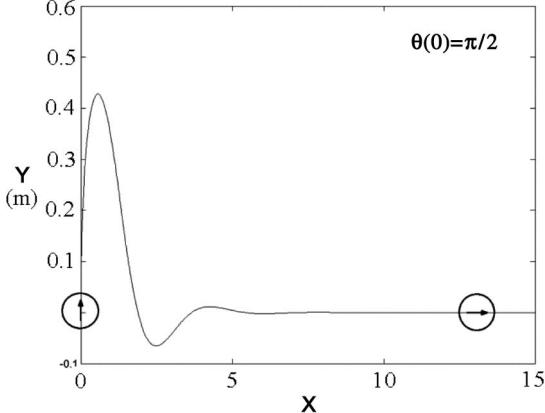
Fig. 12. Trajectories from the nonholonomic kinematic HPF planner.
