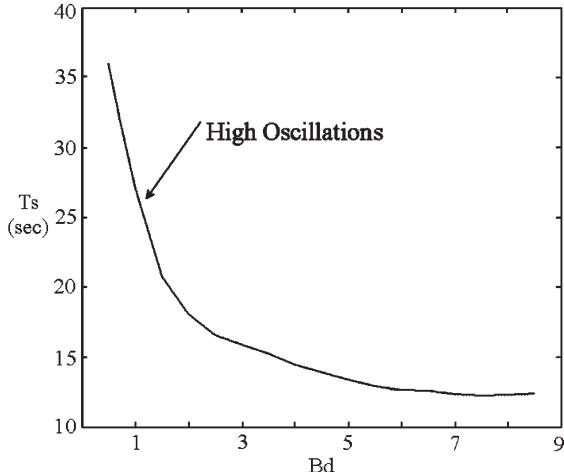
Fig. 8. Settling time versus NADF coefficient.
