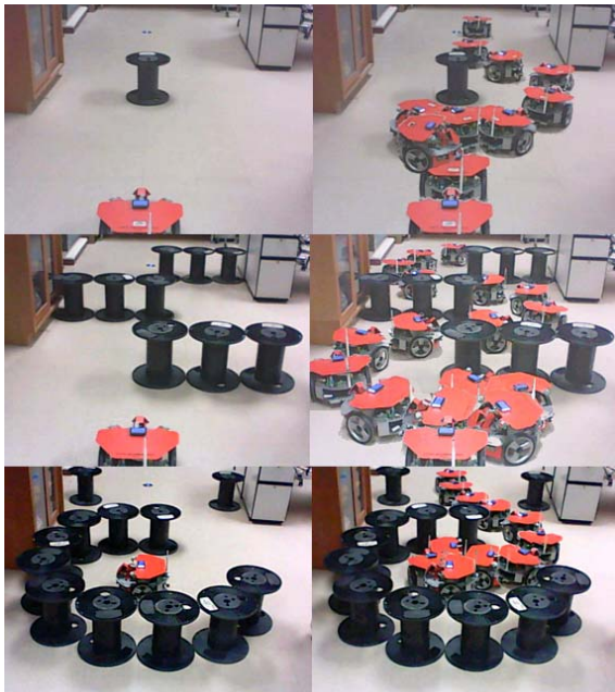
Fig. 10. Trials of X80 moving to a target in an unknown environment
