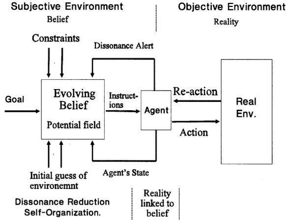
Figure-1: An evolutionary structure for motion planners.
