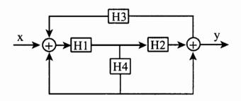
Use the block diagram reduction method to compute the transfer function of the system H=Y/X
