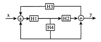
Use the signal flow graph technique to compute the transfer function of the above system H=Y/X
