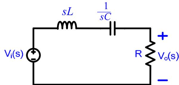
Fig. 38-3 s-domain equivalent for the circuit in Fig. 38-1a
