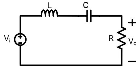
Fig. 38-1a A Series RLC Bandpass filter
