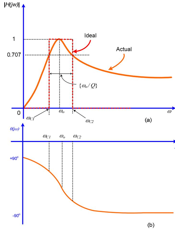
Fig. 38-2 The frequency response plot for the series RLC bandpass filter circuit in Fig. 38-1
