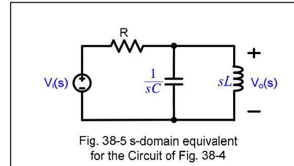
Fig. 38-5 s-domain equivalent for the Circuit of Fig. 38-4
