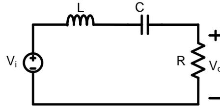
Fig. 38-1a A Series RLC Bandpass filter
