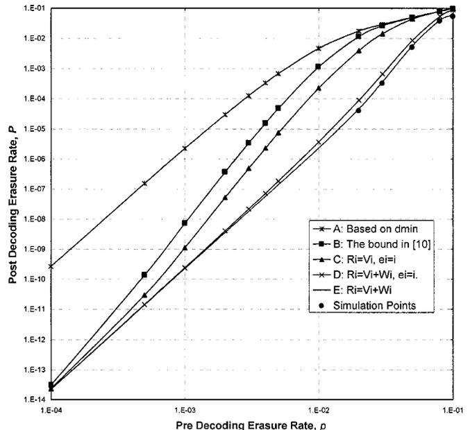
Fig. 3. Various upper bounds on the post-decoding erasure rate of a  $16 \times 16$  SPC product code.
