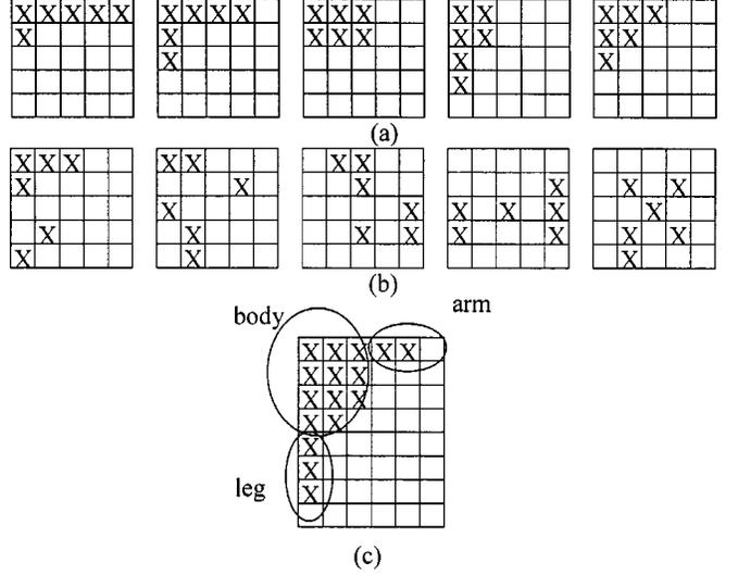
Fig. 2. Illustrative schematics of the proposed approach. (a) Examples of basic patterns of size 6. (b) Examples of patterns generated from the fifth basic pattern in (a). (c) The general structure of an unrecoverable basic pattern (UBP).
