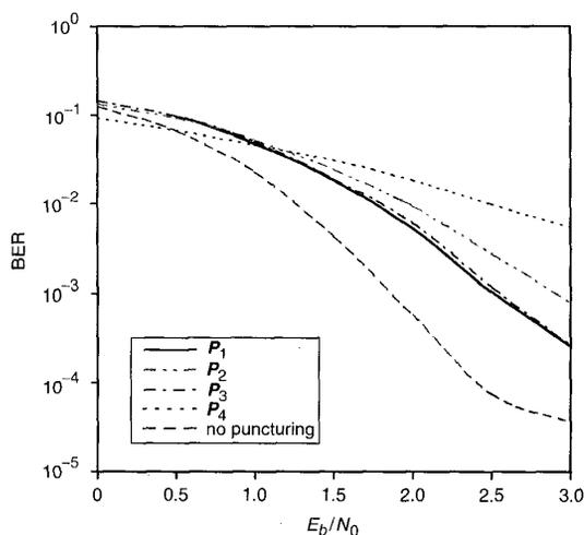
**Fig. 4** Performance of turbo code under different puncturing arrangements of the parity sequence
