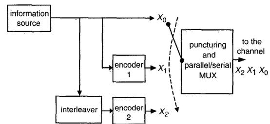
Fig. 1 Simplified turbo-encoder
