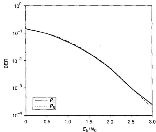
**Fig. 5** Performance under column permutations on the puncturing matrix
