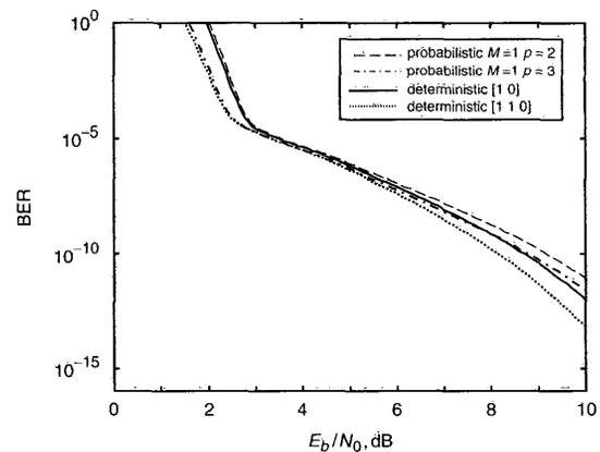
**Fig. 3 Comparison of the upper bounds on the BER using the probabilistic and the deterministic techniques**
