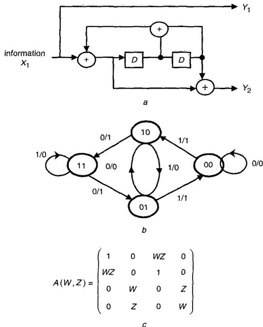
**Fig. 2** Different representations of the (1,5/7) encoder
