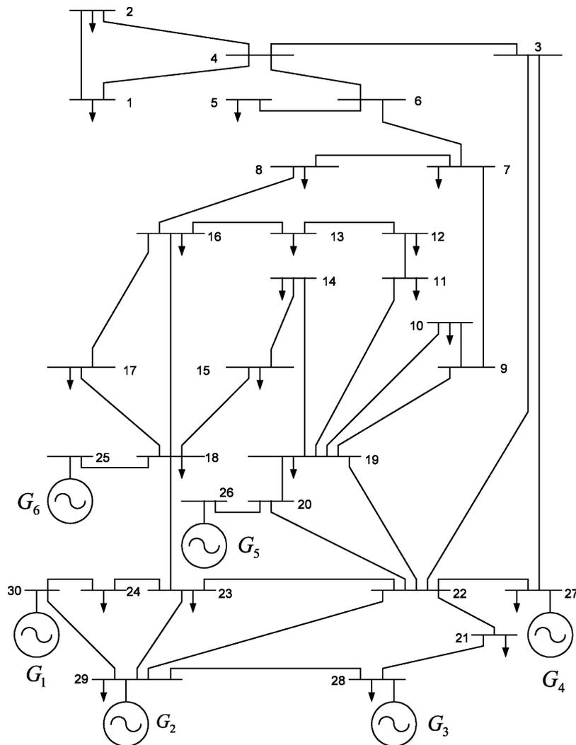
Fig. 3. Single-line diagram of IEEE 30-bus test system.
