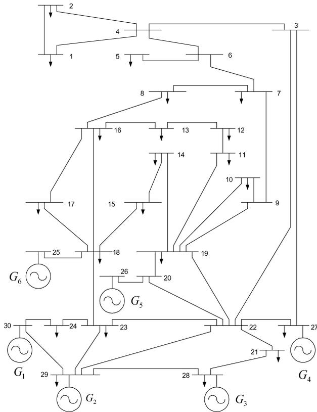
Fig. 2. Single-line diagram of IEEE 30-bus test system.
