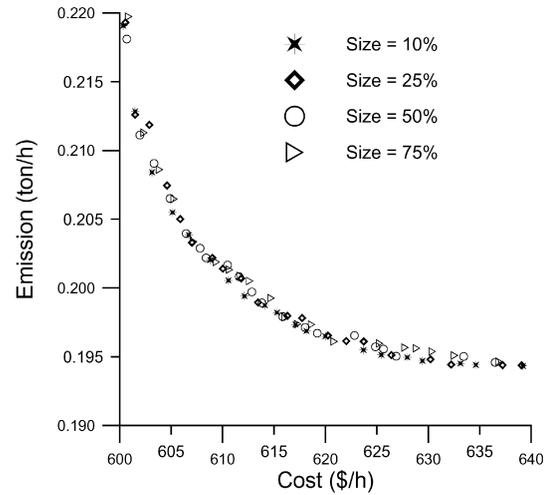
Fig. 3. Effect of the comparison set size on Pareto-optimal front.
