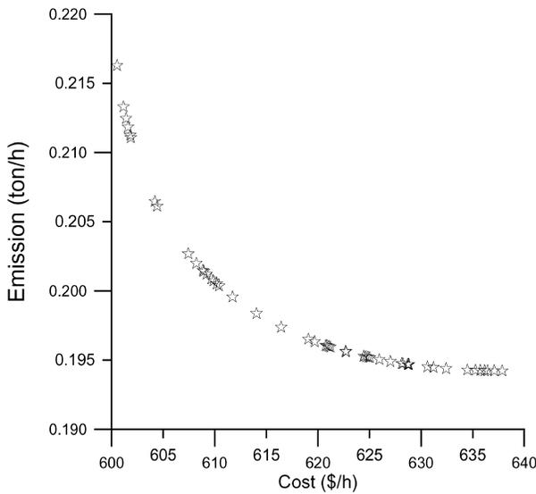
Fig. 5. Pareto-optimal front of objective aggregation in case (a).
