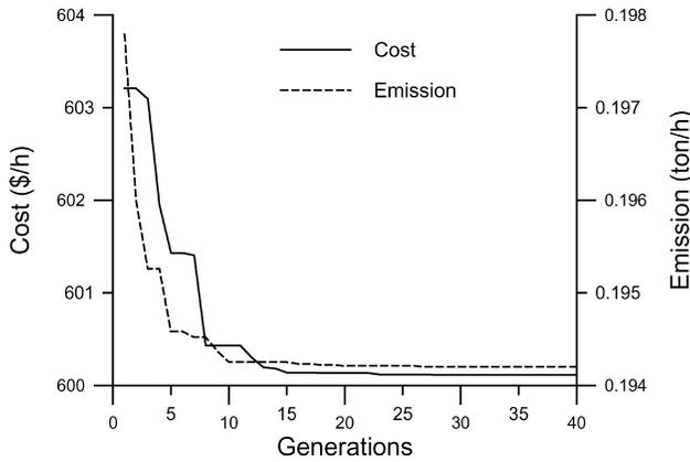
Fig. 4. Convergence of cost and emission objective functions of case (a).
