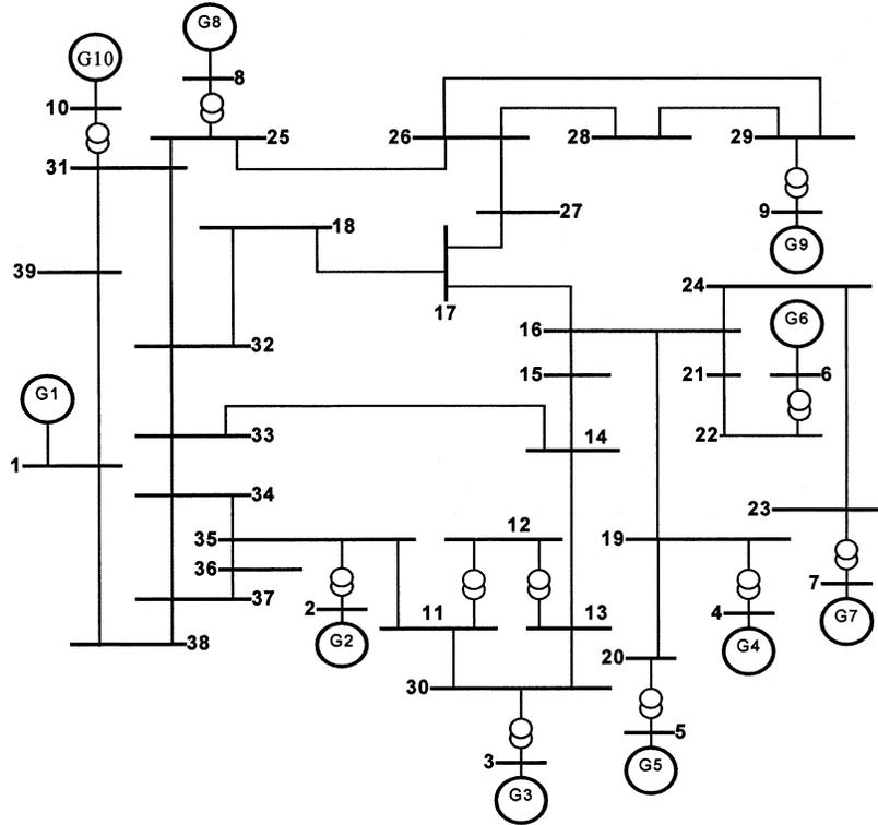
Fig. 2. Single-line diagram for a New England system.
