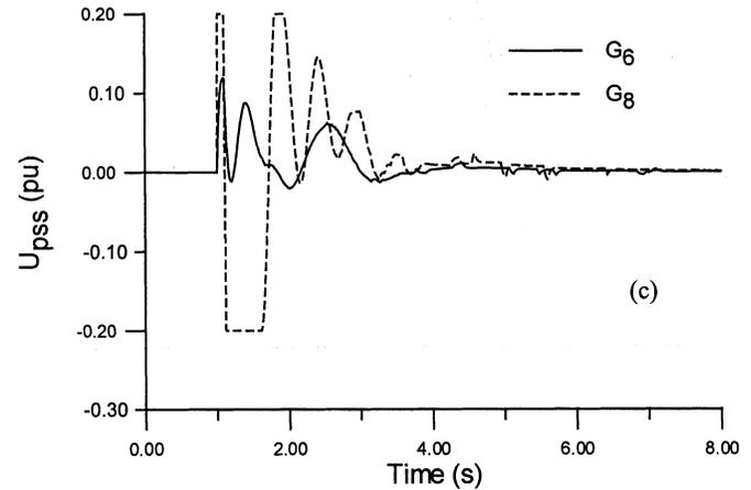
Fig. 4. System responses with the base case.
