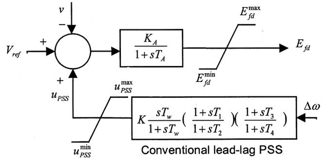
Fig. 1. IEEE-type-ST1 excitation system with conventional lead-lag PSS.
