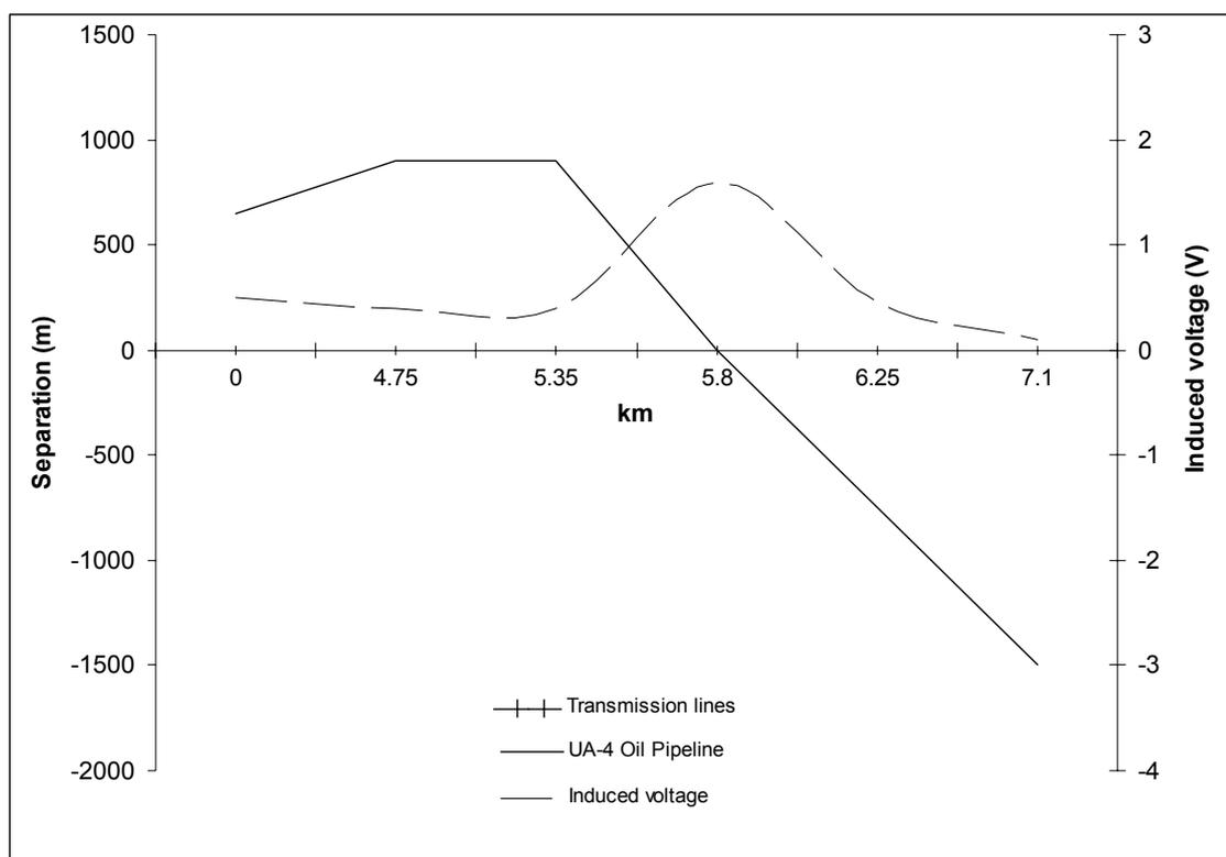
Figure 5.8 Pipeline potential along the axial length of the UA-4 Oil Pipeline
