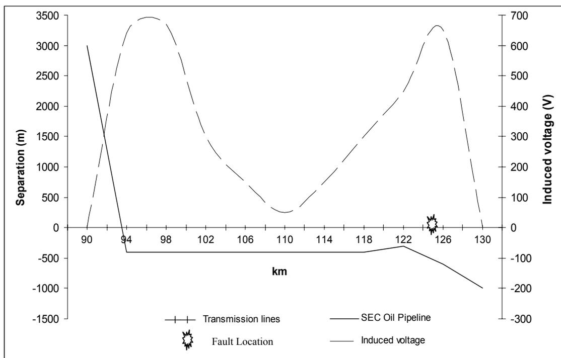
Figure 5.12 Touch voltage along the axial length of the SEC Oil Pipeline
