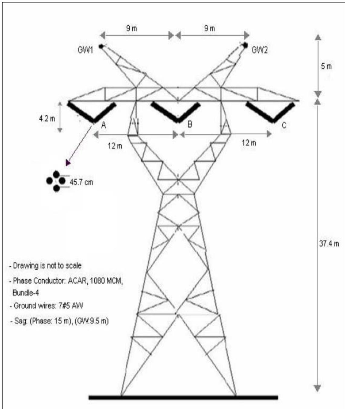
Figure 4.3 Cross section of 380 KV Faras-Qurayyah Transmission Lines
