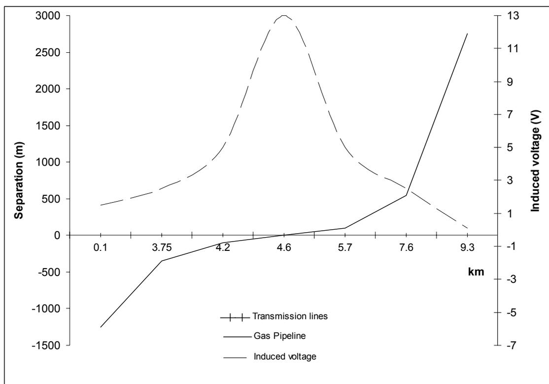
Figure 5.6 Pipeline potential along the axial length of the Gas Pipeline
