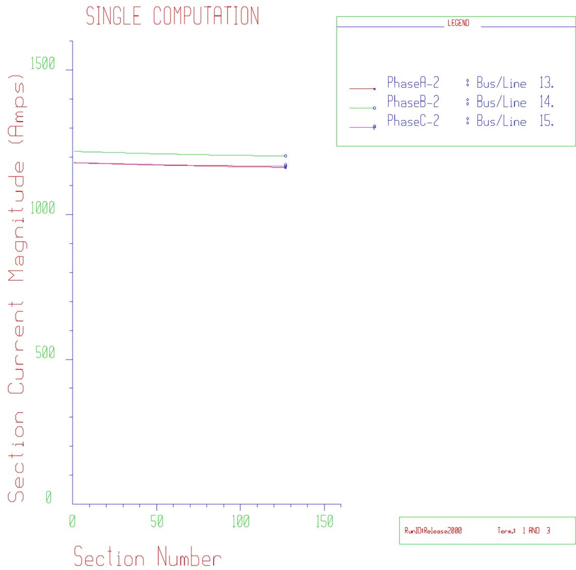
Figure 5.3 The current level on 380KV Shedgum-Qurayyah Transmission Lines
