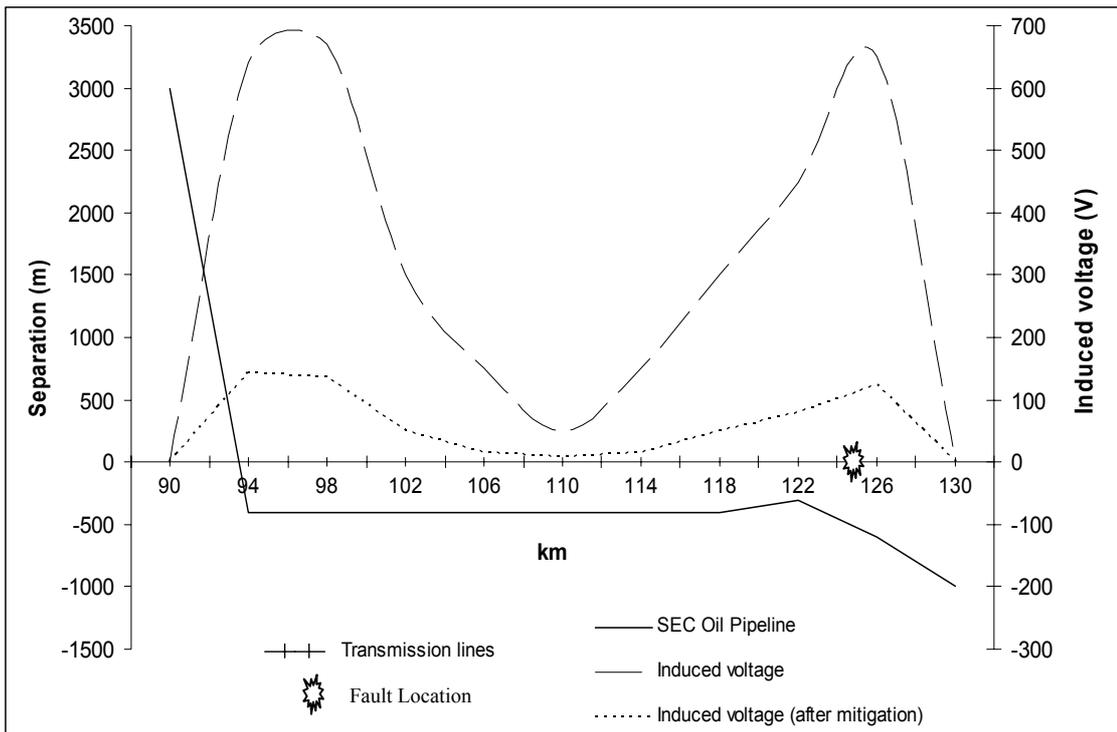
Figure 6.3 Touch voltage along the SEC Oil Pipeline after mitigation
