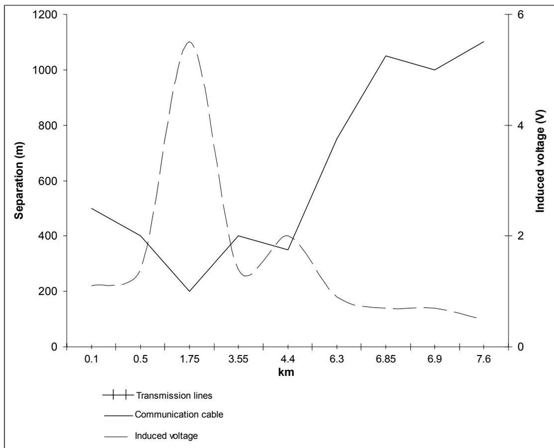
Figure 5.10 Induced voltage along the communication cable
