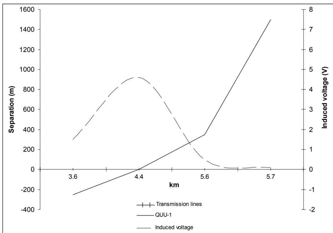
Figure 5.9 Pipeline potential along the axial length of the QUU-1 Pipeline (Case-2)
