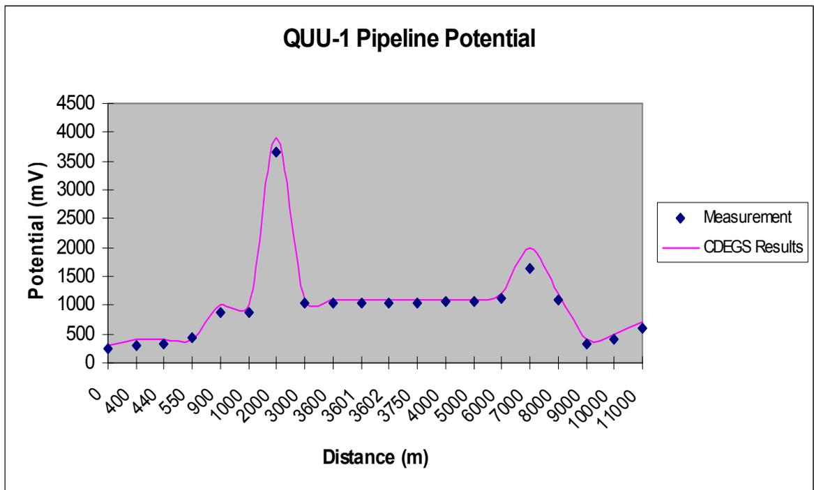
Figure 5.1 Pipeline potential along the axial length of the QUU-1 Pipeline
