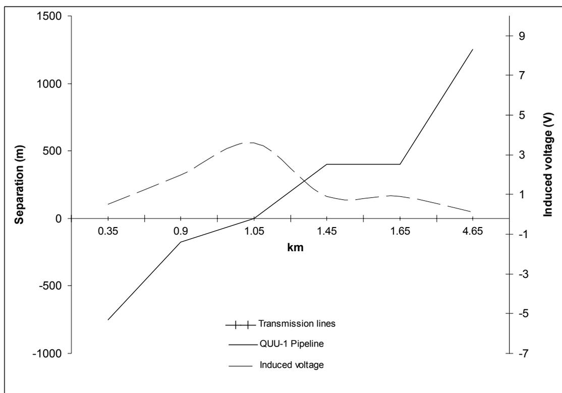
Figure 5.7 Pipeline potential along the axial length of the QUU-1 Pipeline (Case-1)
