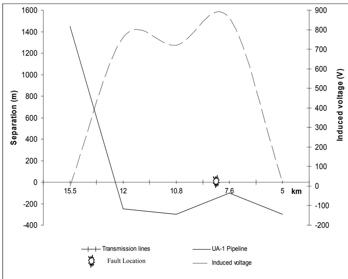
Figure 5.11 Touch voltage along the axial length of the UA-1 Pipeline
