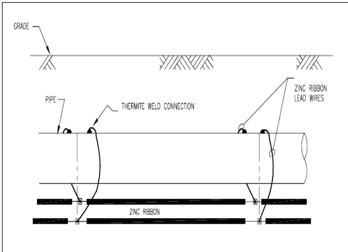
Figure 6.1 Typical gradient control wire installation. [35]
