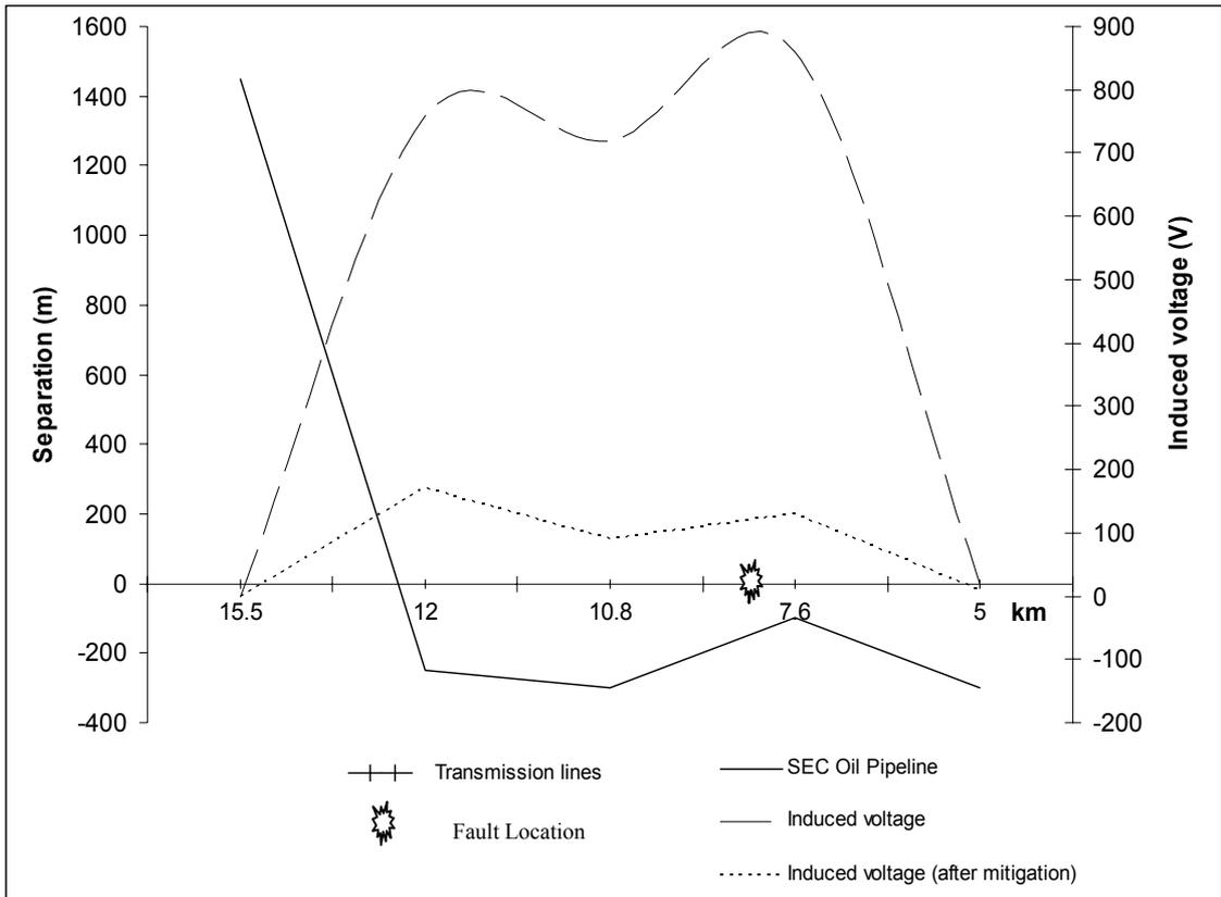
Figure 6.2 Touch voltage along the UA-1 Pipeline after mitigation
