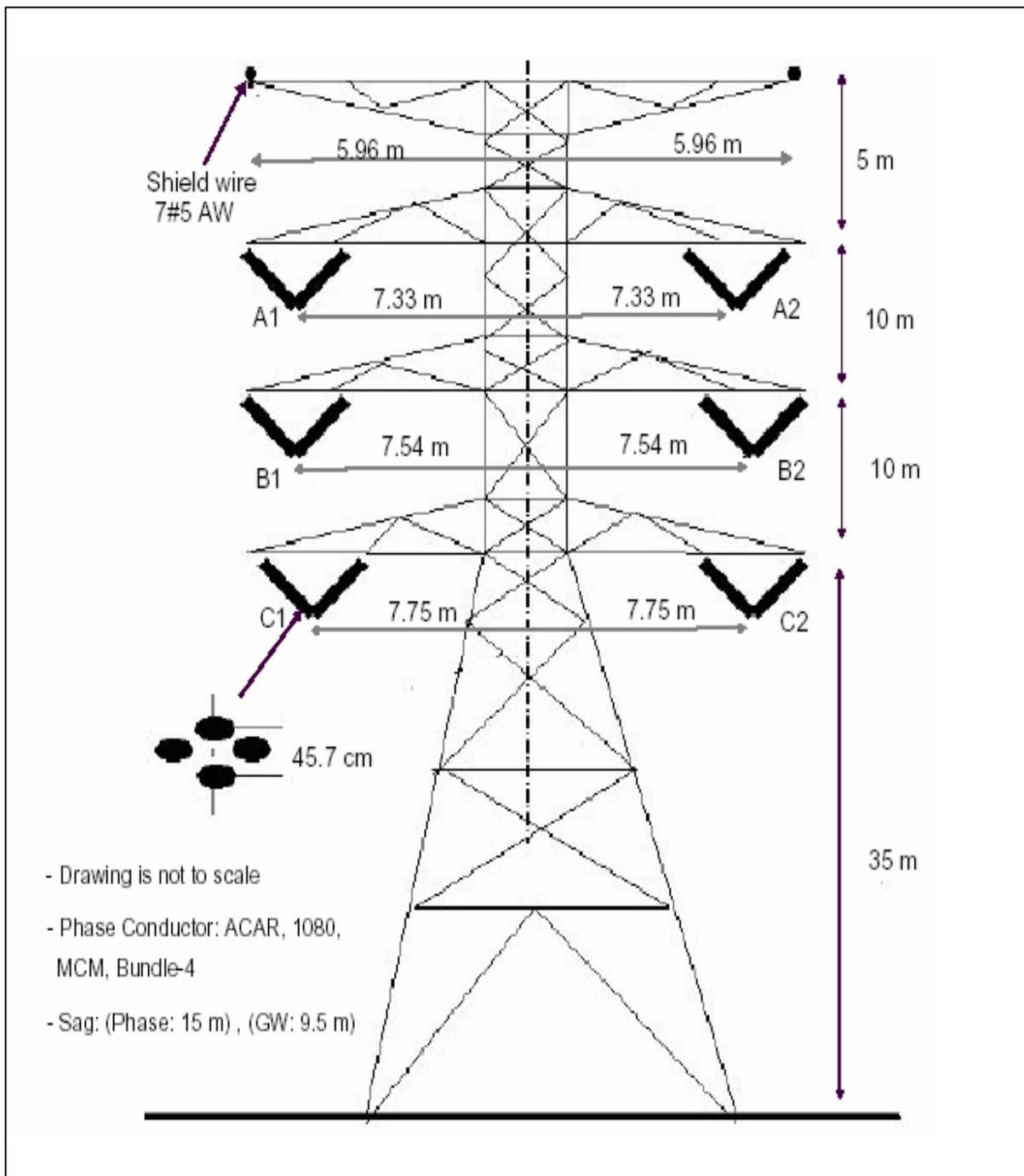
Figure 4.4 Cross section of 380 KV Shedgum-Qurayyah Transmission Lines
