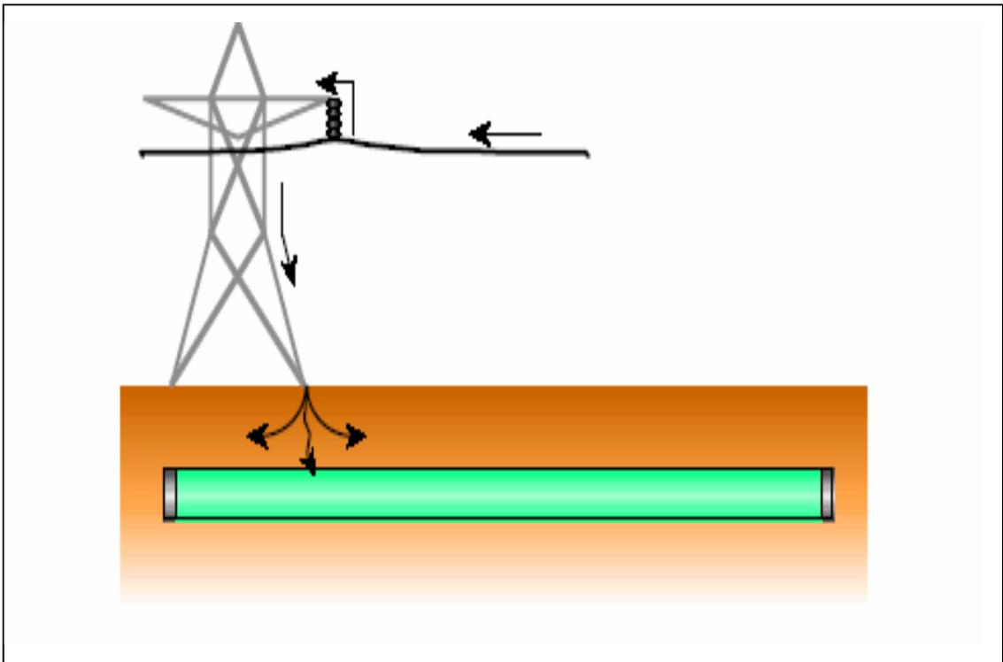
Figure 1.2 Conductive coupling during line-to-ground fault condition. [4]
