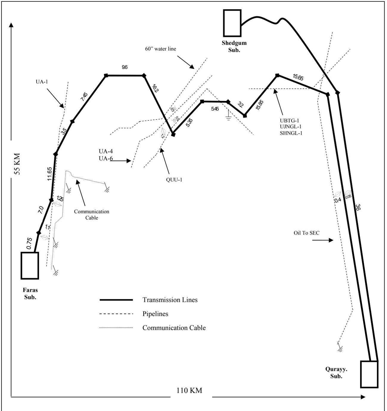
Figure 4.1 380 KV network with buried pipelines & cables to be modeled. (All numbers are in km)
