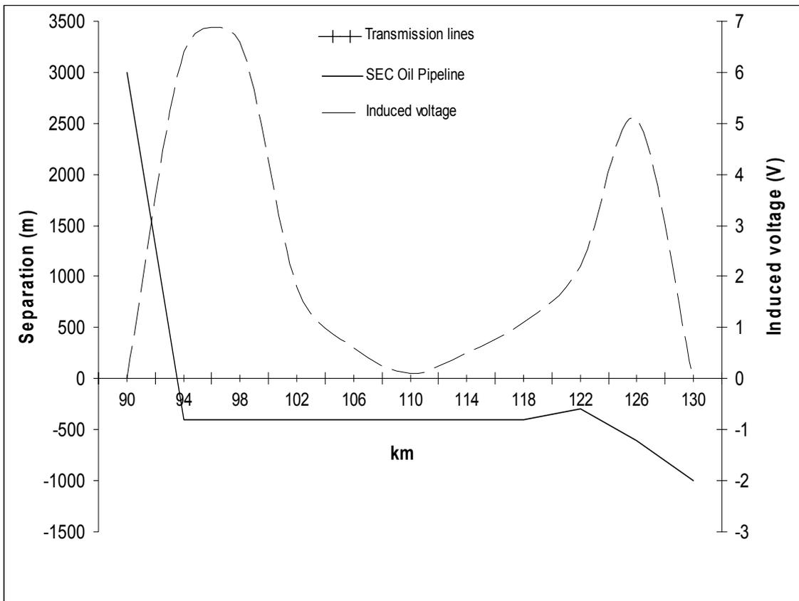
Figure 5.5 Pipeline potential along the axial length of the SEC Oil Pipeline
