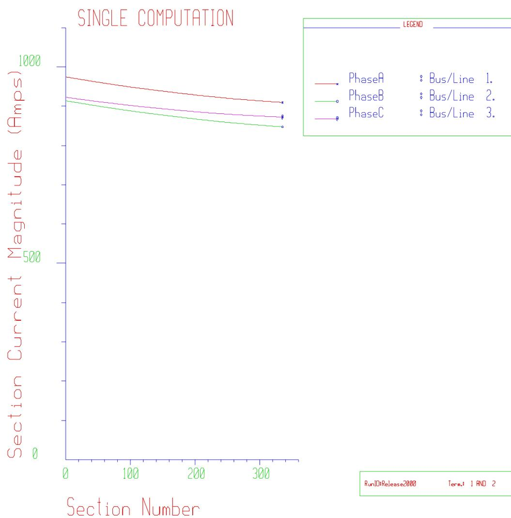
Figure 5.2 Current level on 380KV Faras-Qurayyah Transmission Lines
