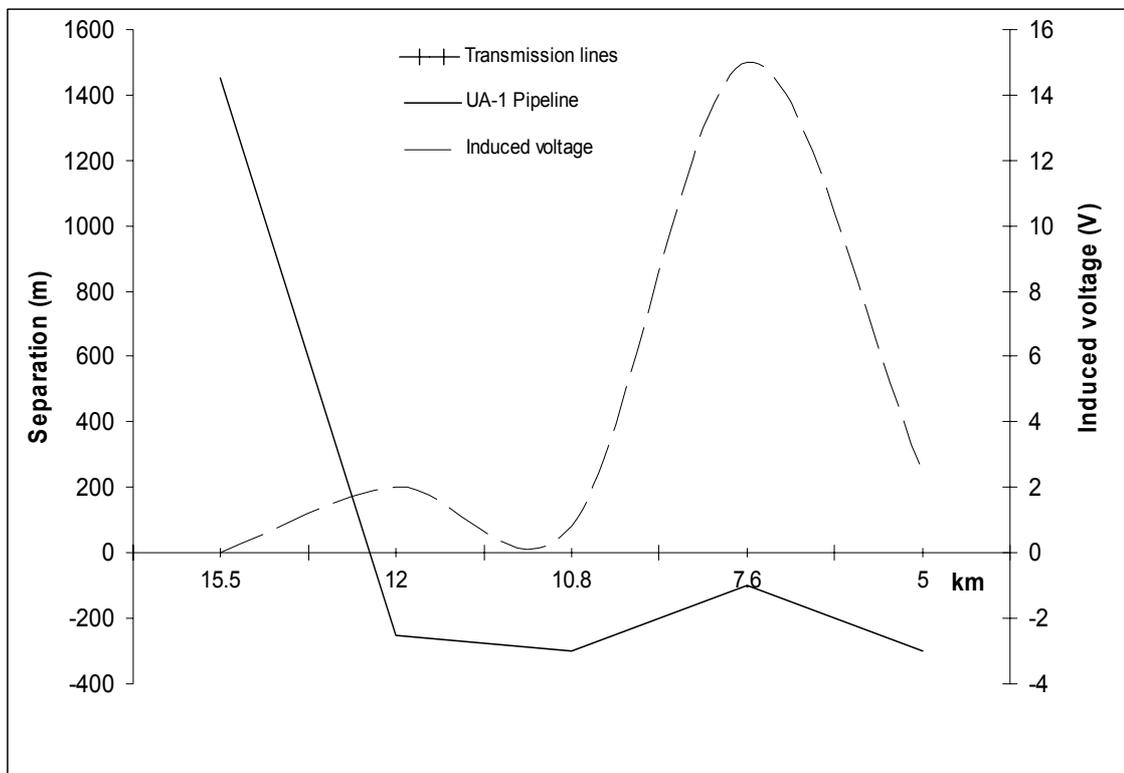
Figure 5.4 Pipeline potential along the axial length of the UA-1 Pipeline
