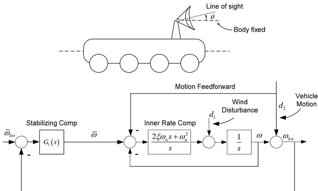
A communication antenna is mounted on a moving vehicle. It is required to precisely regulate the antenna line of sight even though the vehicle is subjected to significant pitching motion and the antenna is subjected to wind loads.
