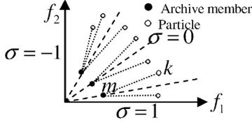
Fig. 1. Finding best local guide for each particle using Sigma method.
