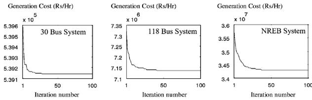
Fig. 3. Convergence characteristics of MOPSO using the selected parameters.
