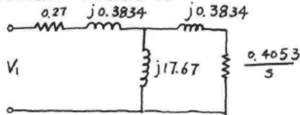
$$(c) \text{ Neglecting } X_m, \quad S_b \approx \frac{R_2'}{\sqrt{R_1^2 + (X_1 + X_2')^2}} = \frac{0.4053}{\sqrt{0.27^2 + 0.7668^2}}$$
