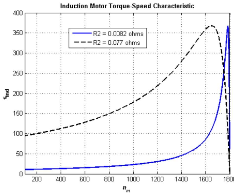
(b) The slip at pullout torque can be found by calculating the Thevenin equivalent of the input circuit from the rotor back to the power supply, and then using that with the rotor circuit model. The Thevenin equivalent of the input circuit was calculated in part (a). The slip at pullout torque is
