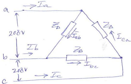
$$(a) \bar{I}_{ab} = \frac{\bar{V}_{ab}}{Z_D} = \frac{208 \angle 30^\circ}{20 \angle -30} = 10.4 \angle 60^\circ A$$
