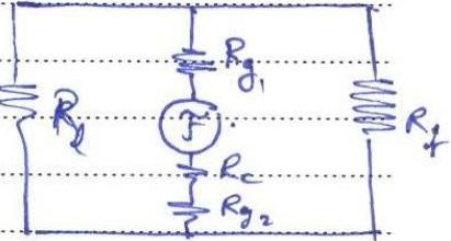
Problem 4: Let  $R_1$  be the reluctance of the left-hand portion of the core,  $R_2$  be the reluctance of the left-hand air gap,  $R_3$  be the reluctance of the right-hand portion of the core,  $R_4$  be the reluctance of the right-hand air gap, and  $R_5$  be the reluctance of the center leg of the core. The total reluctance of the coil is
