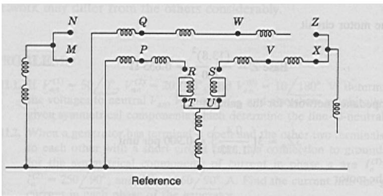
Q. 3) A generator having a solidly grounded neutral and rated 50-MVA, 30-kV has positive-, negative-, and zero-sequence reactances of 25, 15, and 5 percent, respectively. What reactance must be placed in the generator neutral to limit the fault current for a bolted (i.e., solidly grounded) line-to-ground fault to that for a bolted three-phase fault
