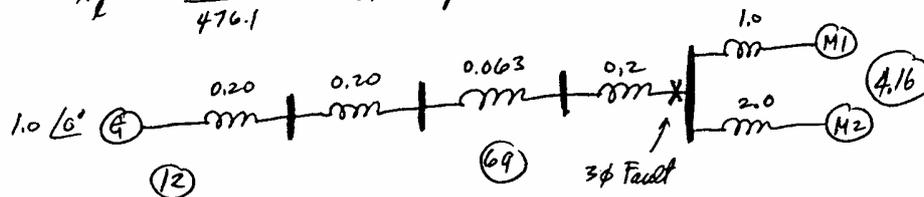
$$\textcircled{b} \quad I_{Fg} = \frac{1.0 \angle 0^\circ}{j(0.2 + 0.2 + 0.063 + 0.2)} = -j1.508 \text{ pu}$$
