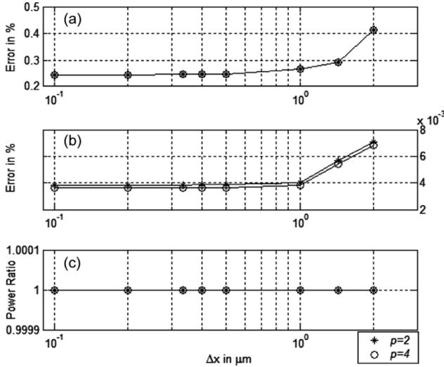
Fig. 2. Convergence of the technique with the spatial step size  $\Delta x$ . (a) The percentage maximum field error. (b) The percentage relative time waist error. (c) The power ratio of the pulsed beams.
