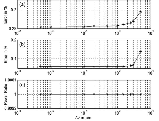
Fig. 1. Convergence of the technique with the longitudinal step size  $\Delta z$ . (a) The percentage maximum field error. (b) The percentage relative spatial waist error. (c) The power ratio of the pulsed beam.
