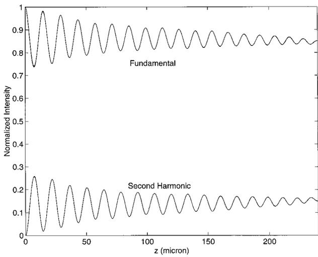
**Figure 3** Normalized intensities of both the fundamental and the second-harmonic fields as a function of the propagational direction inside the nonphase-matched optical waveguide. The input field was excited with an amplitude of  $5 \times 10^9$  and a pulsed first guided mode with an initial pulse width of 100 fs
