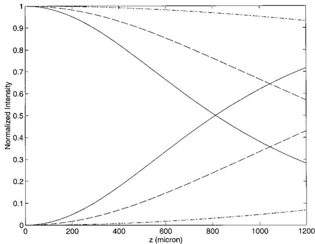
**Figure 4** Normalized intensities of both the fundamental and the second-harmonic fields as a function of the propagational direction inside the phase-matched optical waveguide for different input amplitudes (dashed-dotted is for  $1 \times 10^7$ , dashed is for  $3 \times 10^7$ , and solid is for  $5 \times 10^7$ ) and with an initial pulse width of 150 fs. Curves starting from 1 belong to the *fundamental field*, and curves starting from 0 belong to the *SH field*
