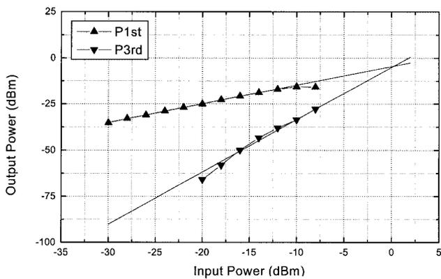
Figure 5 Measurement of IIP3 of the CMOS micromixer
