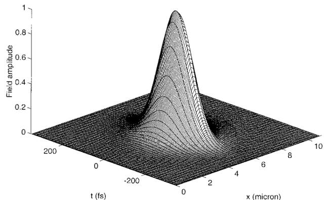
**Figure 2** Three-dimensional plot of the input field used in the analysis, which consists of a pulsed first guided mode with an initial pulse width of 100 fs
