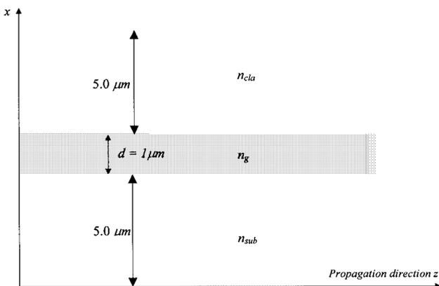
**Figure 1** Two-dimensional slab dielectric waveguide used in the analysis.  $n_{gf} = 1.52$ ,  $n_{sub} = n_{cla} = 1.50$ , and  $\lambda_f = 0.6 \mu\text{m}$
