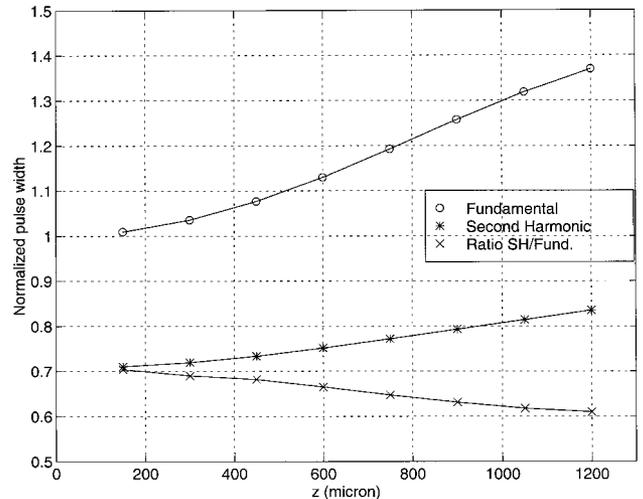
**Figure 6** Fundamental and SH pulse widths as a function of propagation for the phase-matched waveguide. Pulse widths are units of initial pulse width of the fundamental. All parameters are the same as in Figure 5
