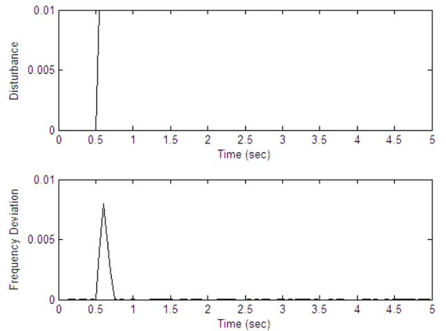
Fig. 8. Frequency Deviation in Single Area with GRC & parameter variation
