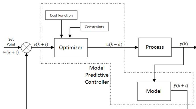
Fig. 1. Structure of MPC
