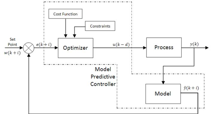
Fig. 1. Structure of MPC
