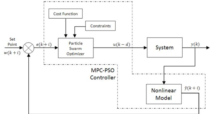
Fig. 3. Structure of Proposed MPC-PSO Controller
