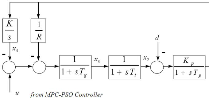
Fig. 4. Block diagram of single area LFC
