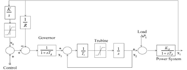
Fig. 7. Block diagram of single area LFC with GRC nonlinearities
