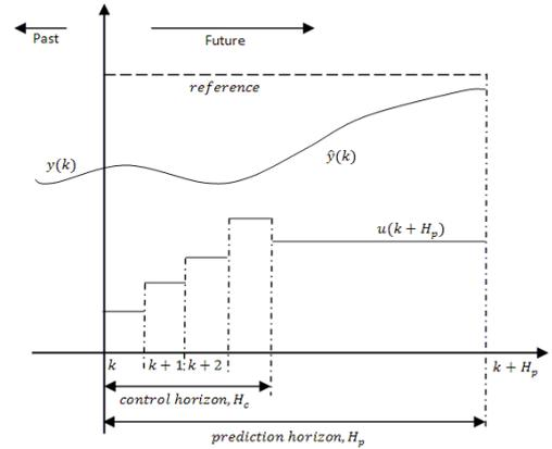
Fig. 2. Predicted output and the corresponding optimal input over a horizon  $H_p$ , where  $u(k)$  is the optimal input,  $\hat{y}(k)$  is the predicted output and  $y(k)$  is the process output.
