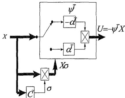
Fig. 1: Block diagram of variable structure controller
