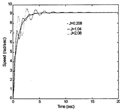
Fig. 6: Effect of inertia constant variations on the speed
