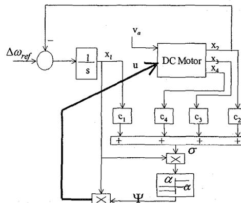
Fig. 3: VSC controller of the field controlled DC motor
