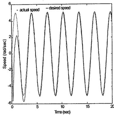
Fig. 5: Actual and desired speed of the DC motor for sinusoidal changes
