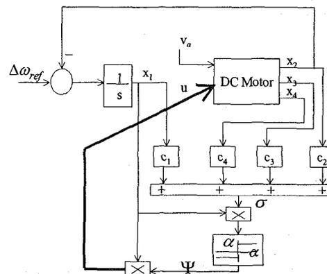
Fig. 3: VSC controller of the field controlled DC motor
