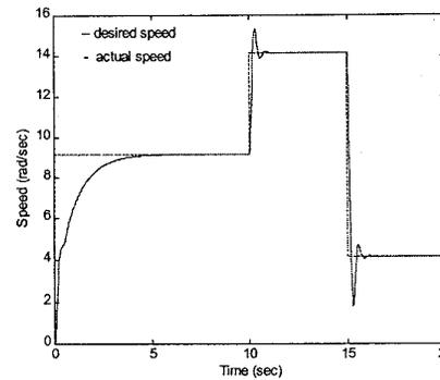
Fig. 8: Actual and desired speed of the DC motor with feedback from ( $x_1$ ) only
