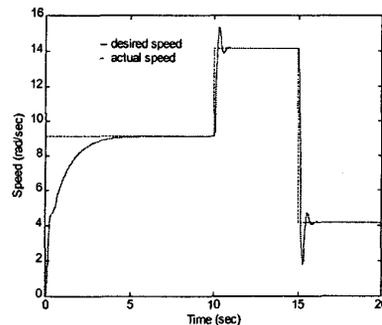
Fig. 4: Actual and desired speed of the DC motor for step changes
