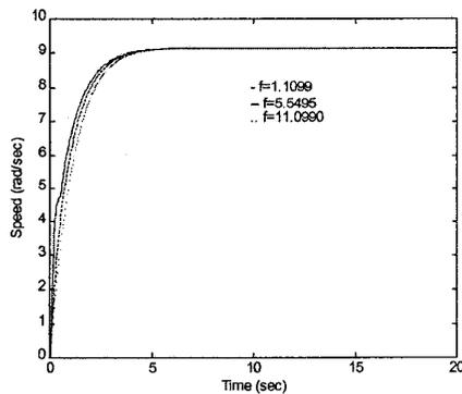
Fig. 7: Effect of friction constant variations on the speed
