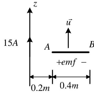
$$\vec{B} = \frac{\mu_0 I}{2\pi\rho} \vec{a}_\phi = \frac{4\pi \times 10^{-7} \times 15}{2\pi\rho} \vec{a}_\phi = \frac{3 \times 10^{-6}}{\rho} \vec{a}_\phi$$
