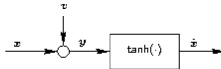
Figure 1.3. Optimal estimation of a BPSK signal embedded in unit-variance additive Gaussian noise.
