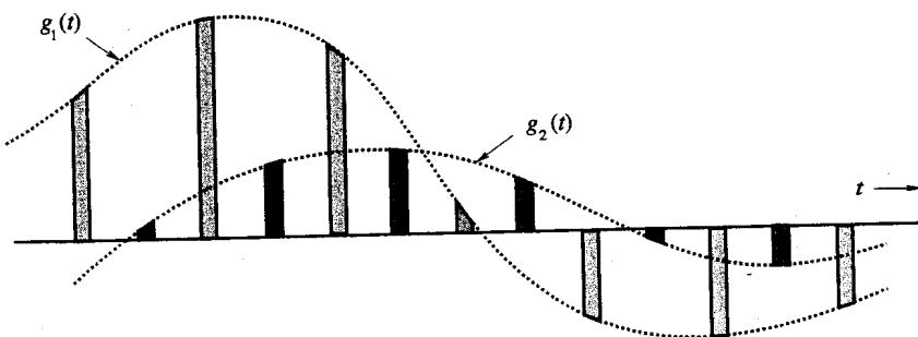
Figure 6.9 Time-division multiplexing of two signals.
