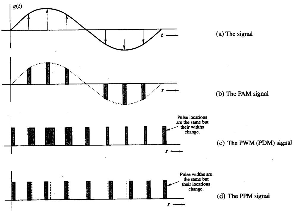
Figure 6.8 Pulse-modulated signals.
