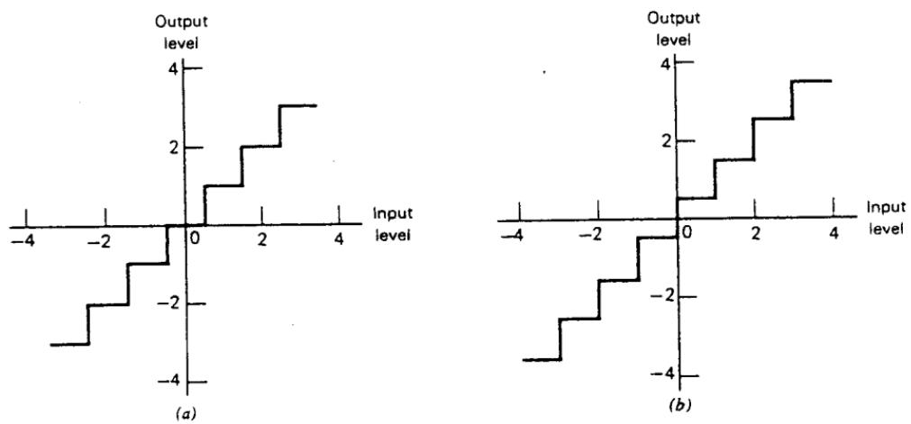
Figure 6.17 Two types of quantization: (a) midtread and (b) midrise.
