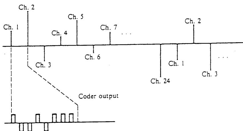
Figure 6.15 T1 carrier system.
