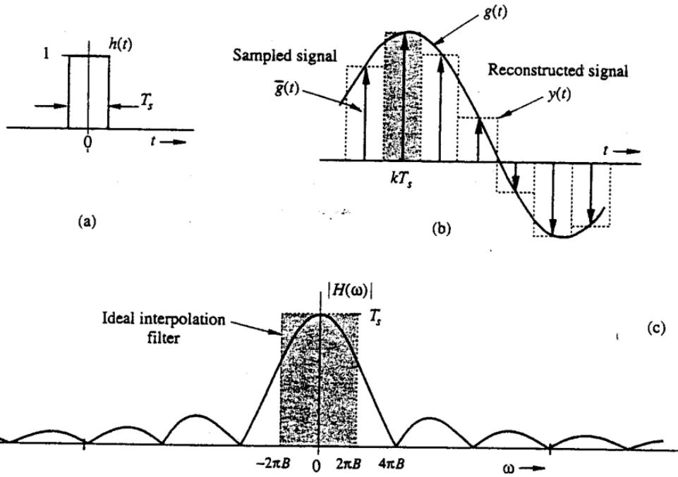
**Figure 6.2** Simple interpolation using zero-order hold circuit.
