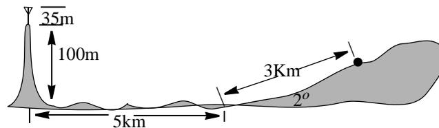
**Figure P-2.14 The geometry of medium sized city built on a quasi-smooth sloping terrain**
