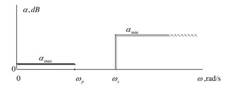
2) (a) Determine (estimate) the degrees necessary for maximally flat and Cauer (elliptic) filters to meet the following requirements.
