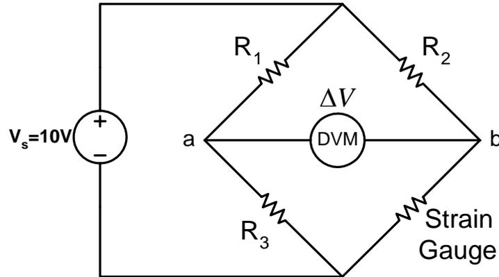
2. Find the voltage difference ( $\Delta V$ ) across nodes “a” and “b” using digital volt-meter (DVM) with no load and record the value in the table.
