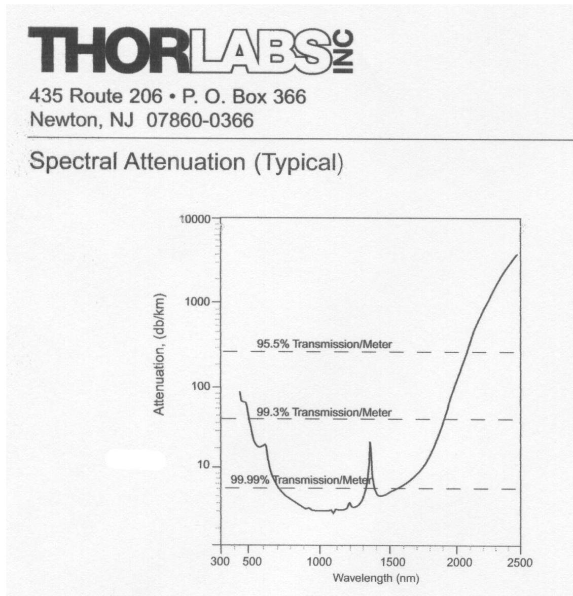
**Figure 5:** Spectral Loss in dB/Km for the Test Fiber (Manufacturer's Data).
