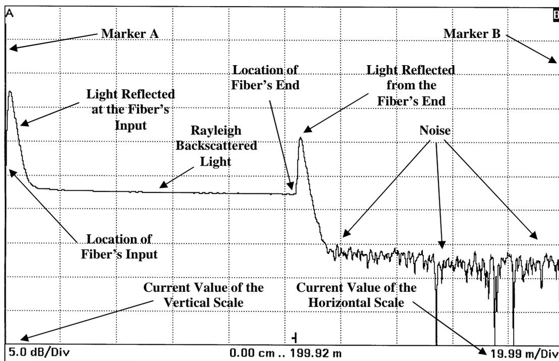
**Figure 6:** OTDR Trace for a 100 Meter long  $50\ \mu\text{m}$  GI fiber Showing Reflected Light from both the Input and Output Fiber's Ends and the Current Locations of Markers A and B. The Trace was Generated at  $\lambda = 0.855\ \mu\text{m}$ .
