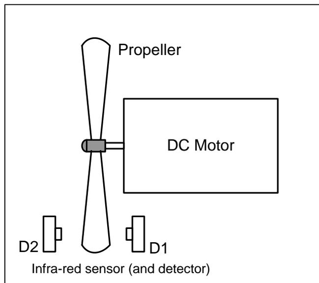
As the motor rotates, the propeller blades pass between D1, an infra-red source, and D2 an infra-red detector, the change in current through the detector provides a signal 3 times per revolution back to Port A bit 4. However, for this to function, SW4A must be set to 'SPEED'.
