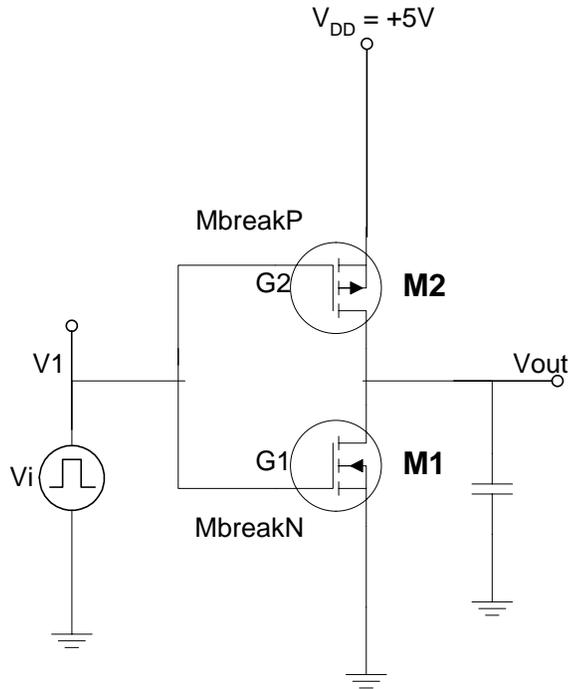
**Figure 1. CMOS Inverter**
