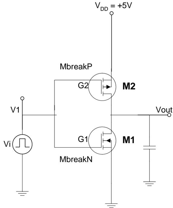
**Figure 1. CMOS Inverter**
