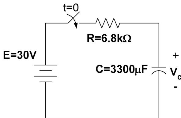
Figure 3: RC circuit for hardware experiment
