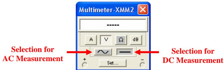
Figure 15: Multimeter properties window
