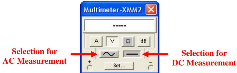
Figure 15: Multimeter properties window
