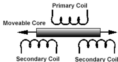
The LVDT is constructed with two secondary coils placed symmetrically on either side of a primary coil contained within the hollow cylindrical shaft. Movement of the magnetic core causes the mutual inductance of each secondary coil to vary relative to the primary, and thus the relative voltage induced from the primary coil to the secondary coil will vary as well.
