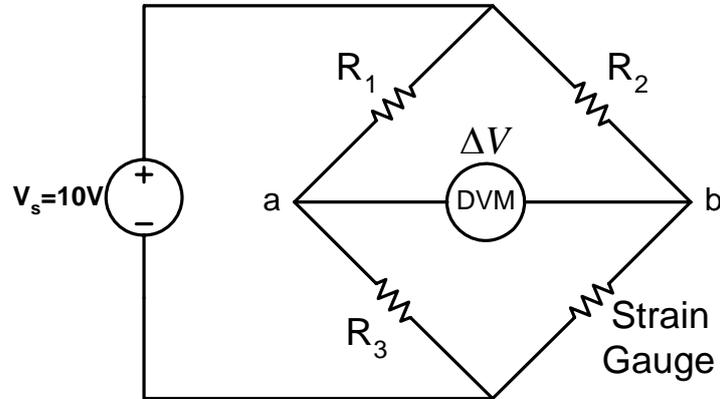
2. Find the voltage difference ( $\Delta V$ ) across nodes “a” and “b” using digital volt-meter (DVM) without any displacement and record the value in the table 2.
