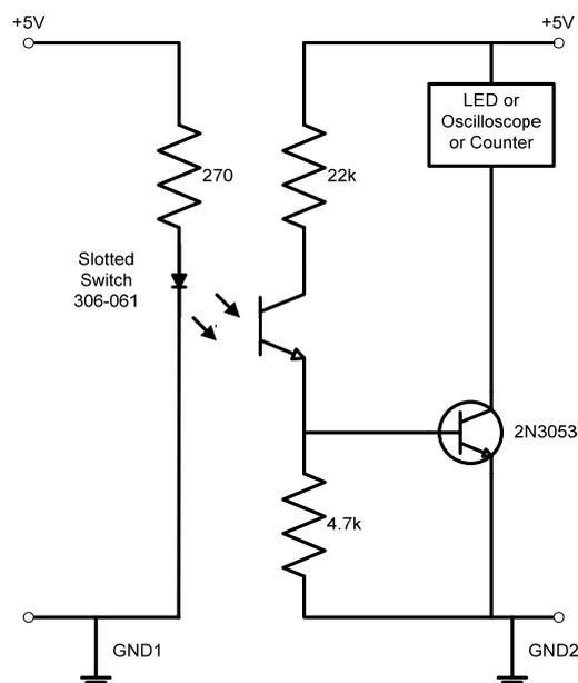
2. First connect the LED at the counting terminal of the circuit.
