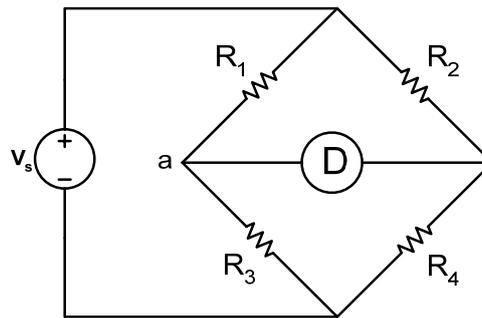
Figure 1: Bridge Circuit.
