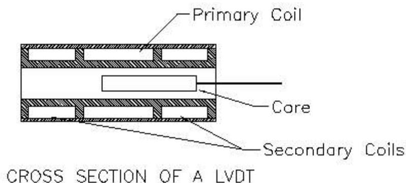
The LVDT is constructed with two secondary coils placed symmetrically on either side of a primary coil contained within the hollow cylindrical shaft. Movement of the magnetic core causes the mutual inductance of each secondary coil to vary relative to the primary, and thus the relative voltage induced from the primary coil to the secondary coil will vary as well.
