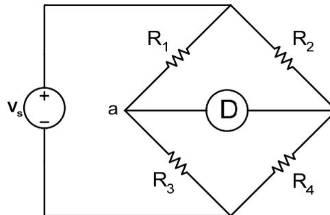
Figure 1: Bridge Circuit.
