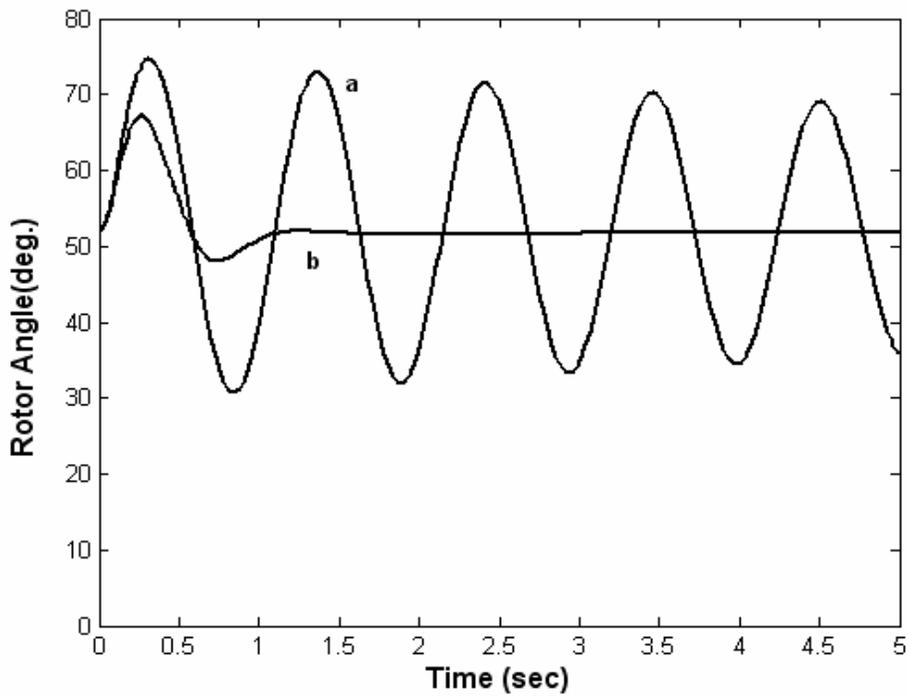
Fig.9 Generator rotor angle variation following a 50% input torque pulse for 0.1sec with, (a) no control, (b) proposed robust damping controller.
