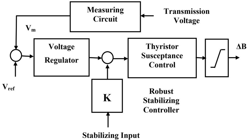
Fig.2 SVC controller block diagram
