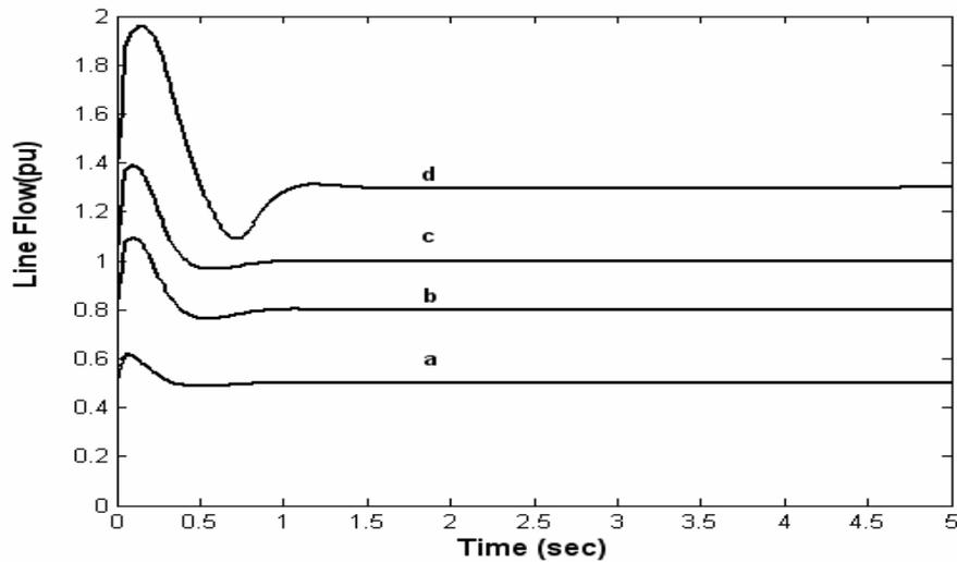
Fig. 14 The real power flow in the line with robust controller following the fault condition corresponding to Fig. 12.
