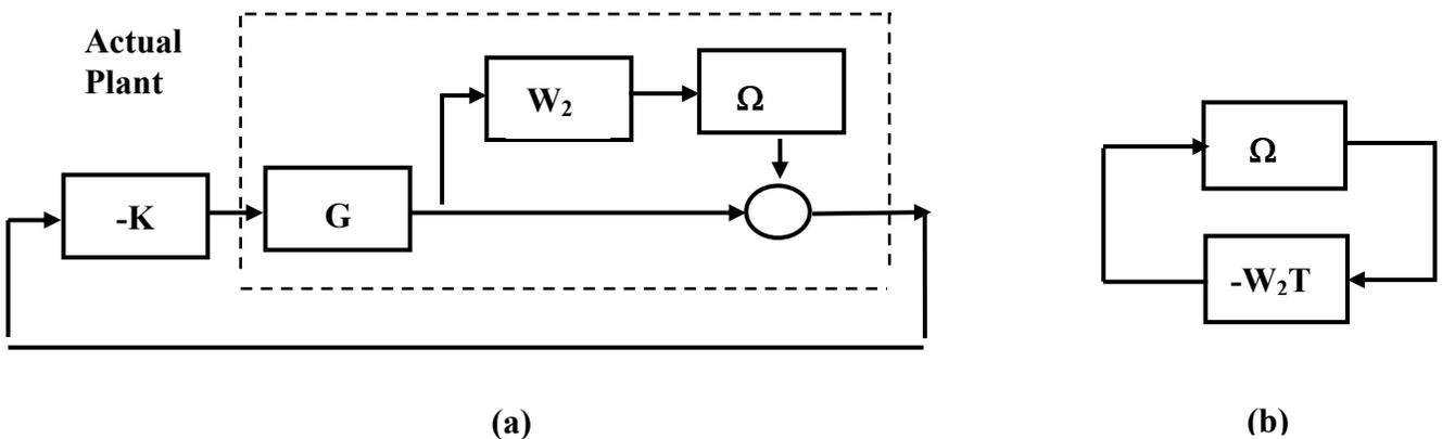
Fig.3 Stability robustness for multiplicative uncertainty at plant output
