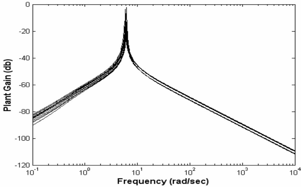
Fig. 5 Bode magnitude diagram of nominal and perturbed plant functions
