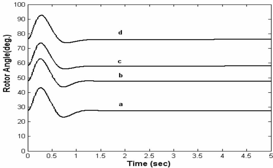
Fig.10 Rotor angle characteristics with the robust damping controller for (a) 0.5 pu output at 0.85 lagging pf, (b) 0.8 pu power at 0.9 pf lag, (c) 1pu power at 0.85 pf, and (d) 1.3 pu power at 0.95 pf lagging.
