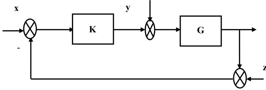
Fig.4 Unity feedback plant with controller.
