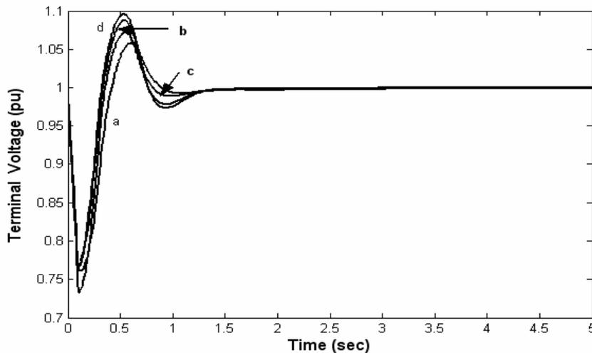
Fig. 11 Terminal voltage variations of the generator corresponding to Fig. 9
