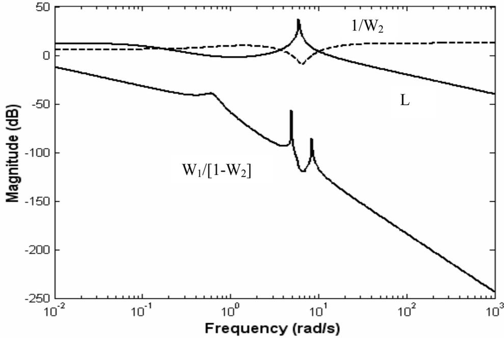
Fig. 7 The loop-shaping boundary plots
