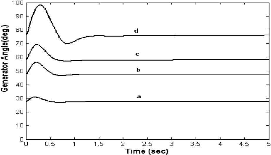
Fig. 12 Generator rotor angle variations with the robust controller following a three-phase fault for, a) 0.5 pu power output at 0.85 pf lag, b)0.8 pu at 0.9 pf lag, c)1pu at 0.85 pf lag and, d)1.3 pu at 0.95 lagging pf.
