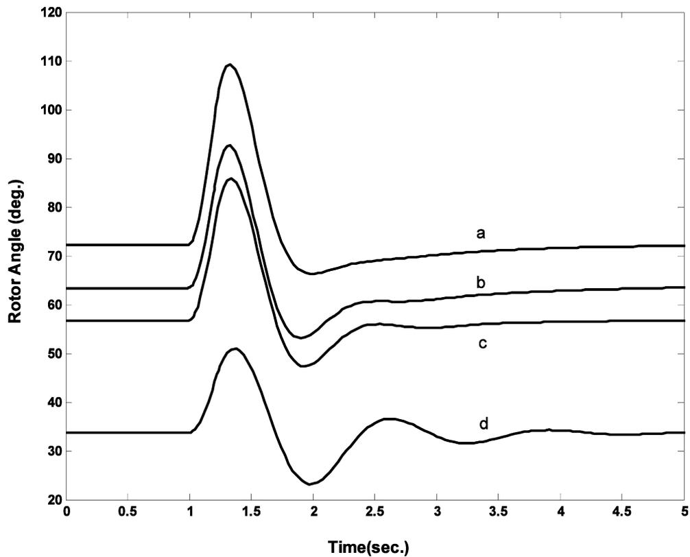
Fig. 13. Generator rotor angle variation following a three-phase fault on the remote bus for 0.1 s with, (a) 1.2 pu power output; (b) 1 pu output; (c) 0.9 pu output and; (d) 0.5 pu output.
