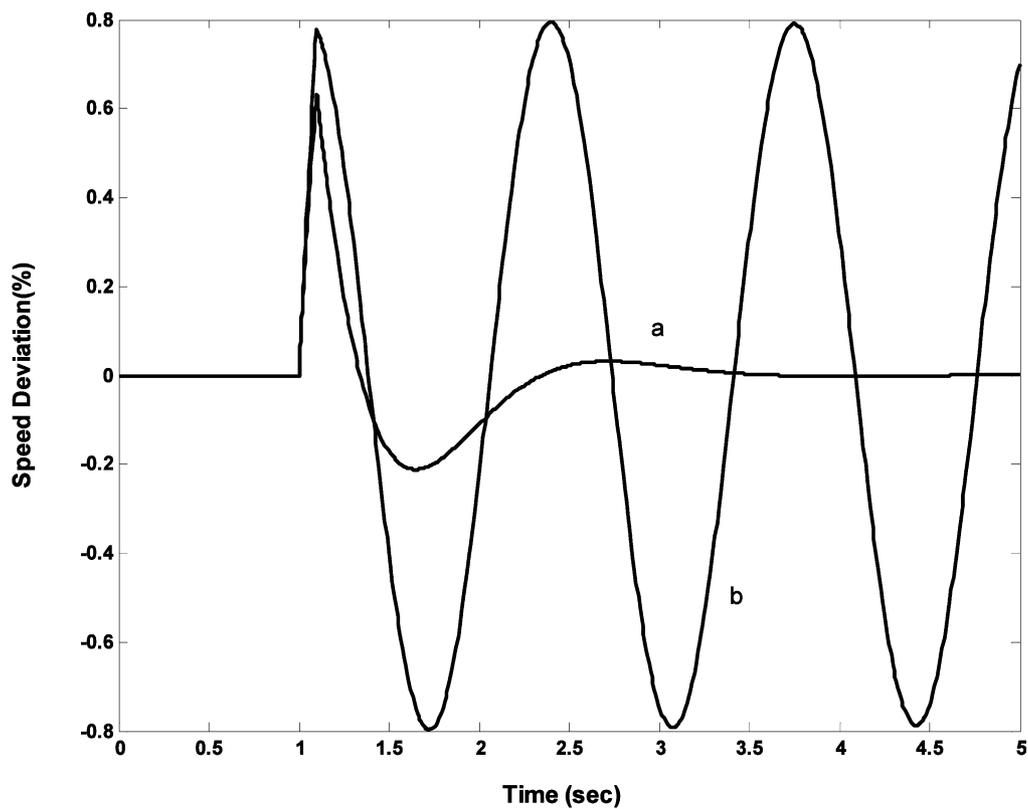
Fig. 9. Generator angular frequency variation corresponding to Fig. 8 with, (a) robust control; and (b) no control.
