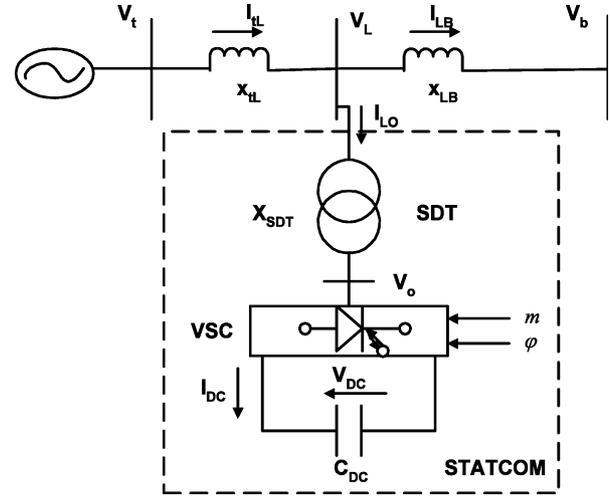
Fig. 1. The single machine infinite bus power system with STATCOM.
