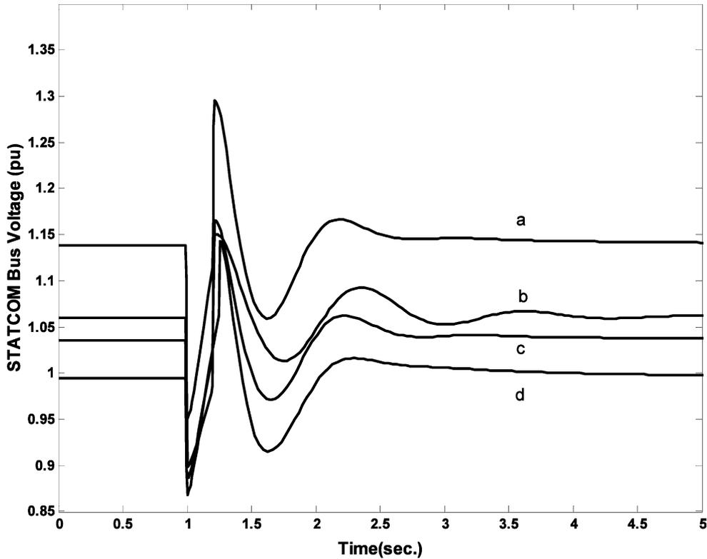
Fig. 14. STATCOM bus voltage variations following the three-phase fault condition of Fig. 13.
