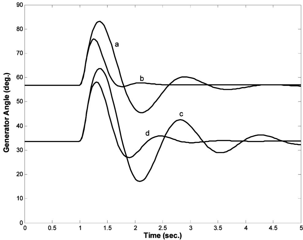
Fig. 15. Comparison of rotor angle characteristics with PID and robust controllers—at nominal loading (a) PID control; (b) robust control; at 0.5 loading; (c) PID control; (d) robust control.
