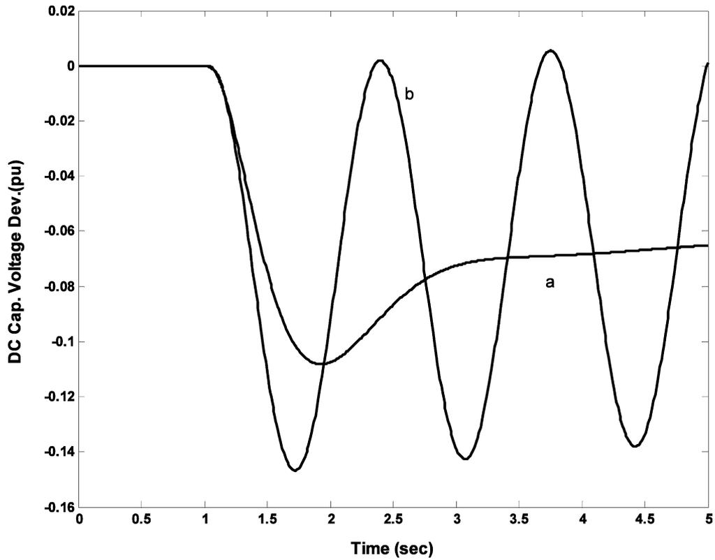
Fig. 10. D.C. capacitor voltage variation corresponding to the disturbance condition of Fig. 8 with, (a) robust control; and (b) no control.
