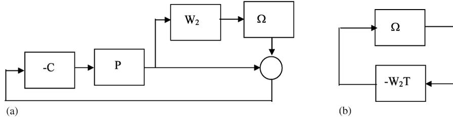
Fig. 4. (a) Feedback loop with uncertainty representation; (b) feedback loop in standard reduced form.
