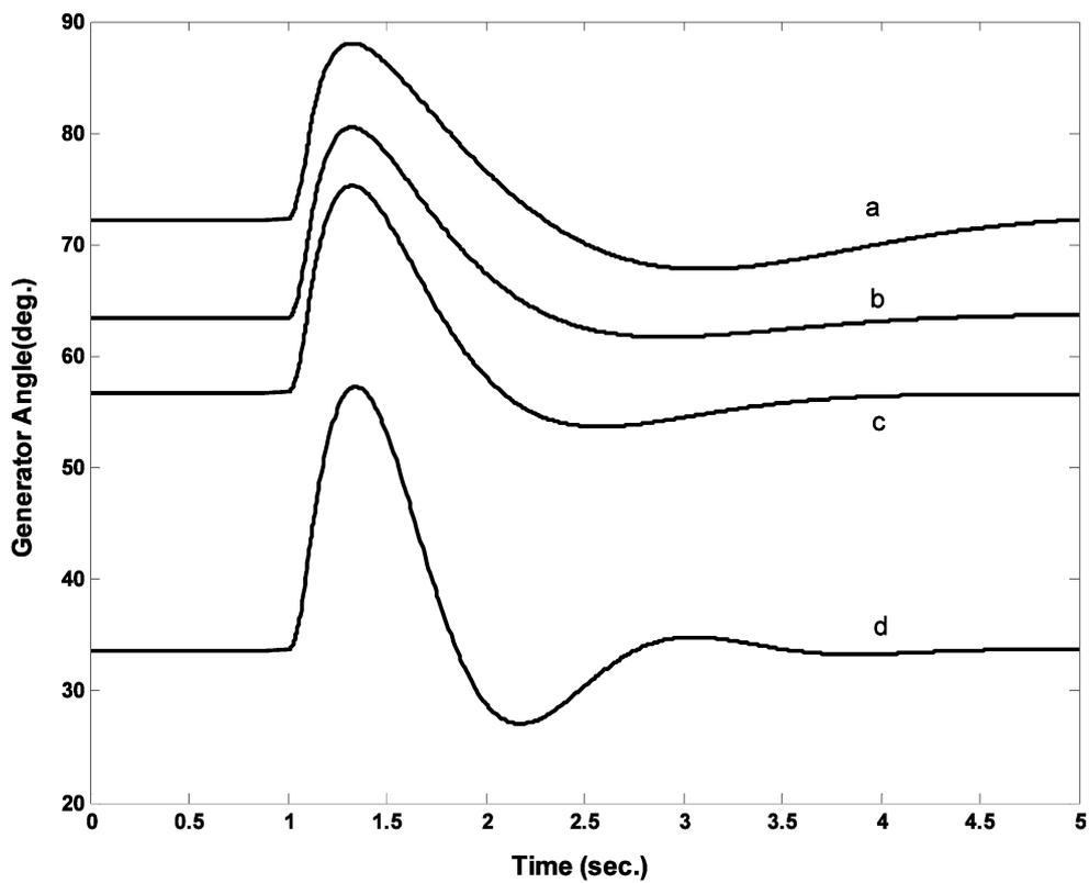
Fig. 11. Generator angle variations following 50% input torque pulse for 0.1 s, for (a) 1.2 pu power output, (b) 1 pu output, (c) 0.9 pu output, and (d) 0.5 pu output.
