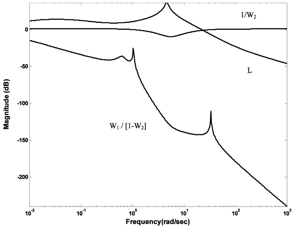
Fig. 6. Loop-shaping plots relating  $W_1$ ,  $W_2$  and  $L$ .
