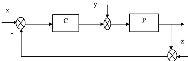
Fig. 3. Unity feedback plant with controller.
