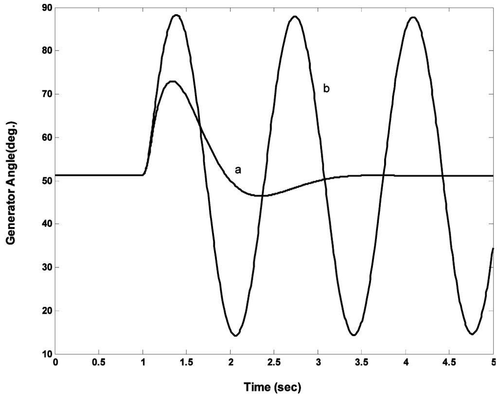
Fig. 8. Rotor angle variation following 50% input torque pulse for 0.1 s with (a) proposed robust control; and (b) no control.
