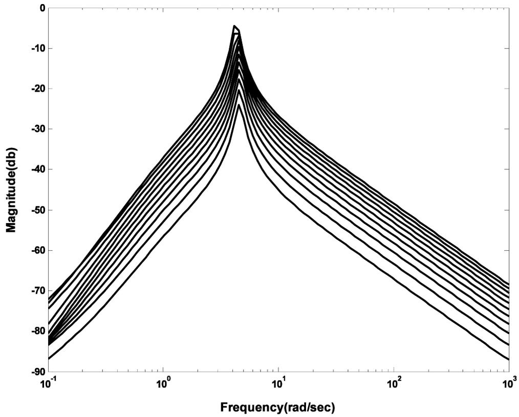
Fig. 5. dB-magnitude plot for nominal and perturbed plant transfer functions.
