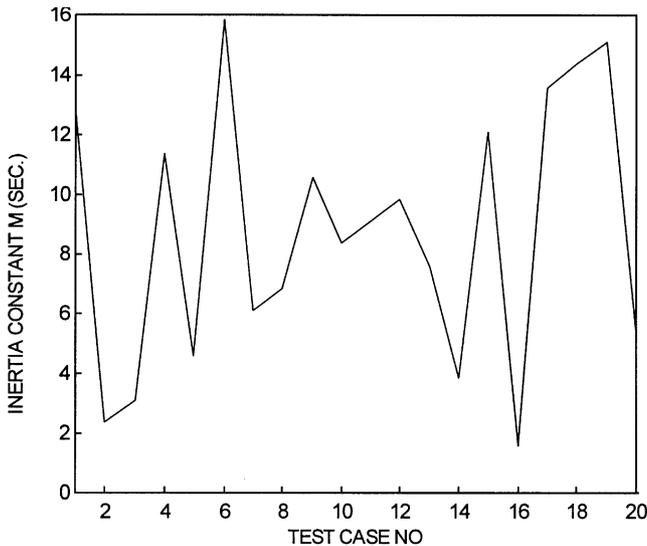
Fig. 12. Inertia constant  $M$  obtained through the RBF network for various test cases (the actual values overlapping with the predicted ones).
