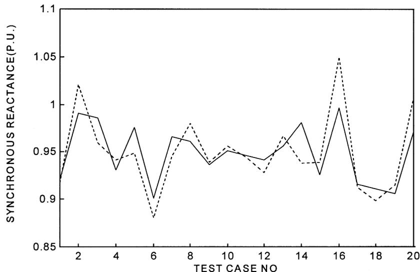
Fig. 8. Comparison of the values of synchronous reactance  $x_d$ , — actual, - - - back-propagation net estimates.
