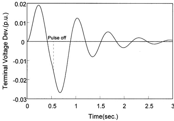
Fig. 5. Terminal-voltage variation of the local generator for the disturbance condition of Fig. 4.
