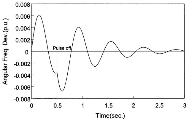
Fig. 4. Angular speed deviation of local generator following a 35% input torque pulse for 0.5 s.
