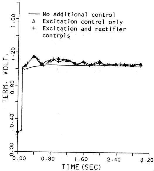
Fig. 7. Terminal voltage variation of generator CD for a 0.1 sec duration fault corresponding to Fig. 3.
