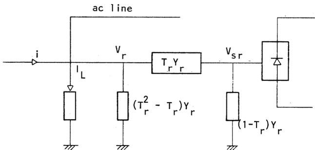
Fig. A2. ACDC rectifier transformer end configuration.
