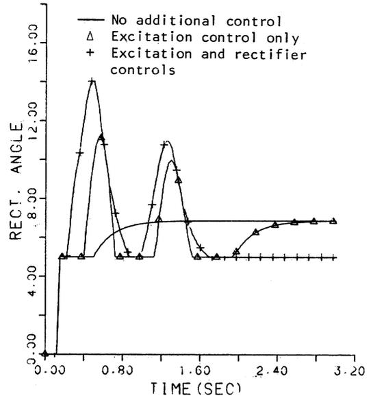
Fig. 8. Rectifier firing angle variation for a three phase fault corresponding to Fig. 3.
