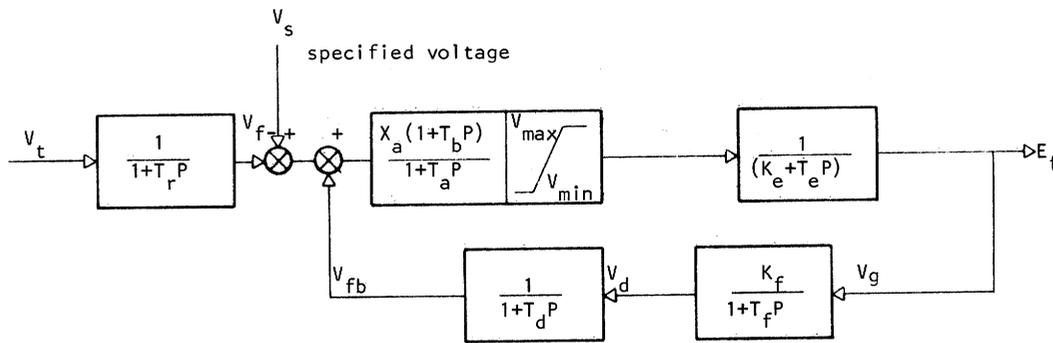
Fig. A1. AVR block diagram.
