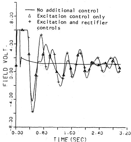
Fig. 5. Field voltage variation of generator CD corresponding to fault conditions of Fig. 3.
