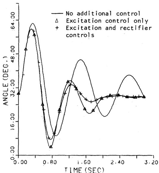
Fig. 4. Rotor angle variation of generator CD (lumped) for 0.1 sec duration fault corresponding to Fig. 3.
