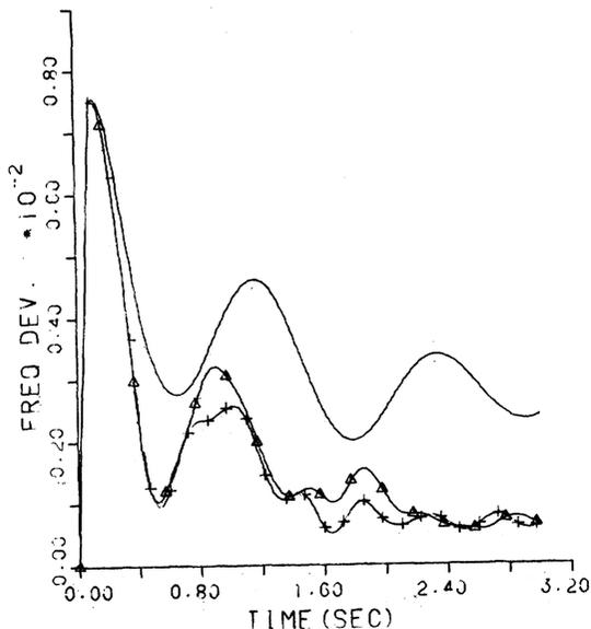
Fig. 3. Normalized frequency deviation characteristics for a three phase fault of 0.1 sec duration on generator bus CD. Responses are with (a) No control (no symbol), (b) with excitation control alone ( $\Delta$ ) and (c) with excitation and rectifier firing control (+).
