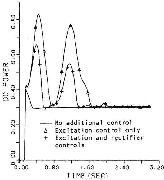
Fig. 6. Transient power flow on the DC line for a 0.1 sec duration fault corresponding to Fig. 3.
