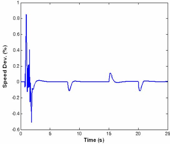
Fig. 4. Speed deviation of the generator with adaptive pole-shift control
