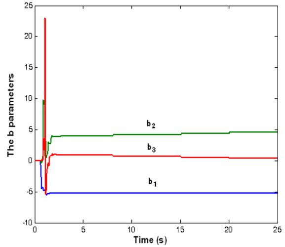
Fig. 7. The variation of the b-parameters of the adaptively identified plant function
