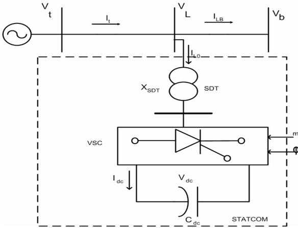
Fig. 1. A single machine system with STATCOM
