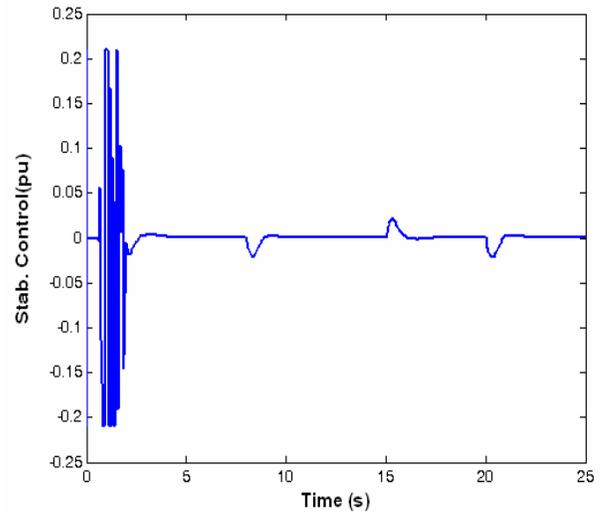
Fig. 8. Control signal produced by the adaptive process
