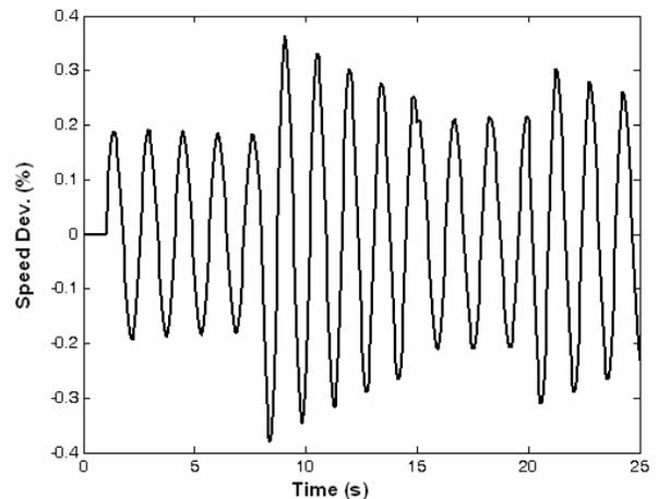
Fig. 3. Generator speed deviation when excited with alternate torque steps
