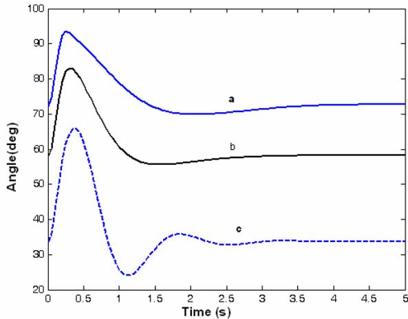
Fig. 9. Generator rotor angle variations with the proposed pole-shift control for the loadings of a)1.2 pu, b) 0.9 pu, and c) 0.5 pu. The disturbance considered is a 50% torque pulse for 0.1s
