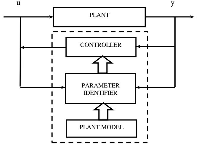
Fig. 2. Block diagram of self-tuning controller
