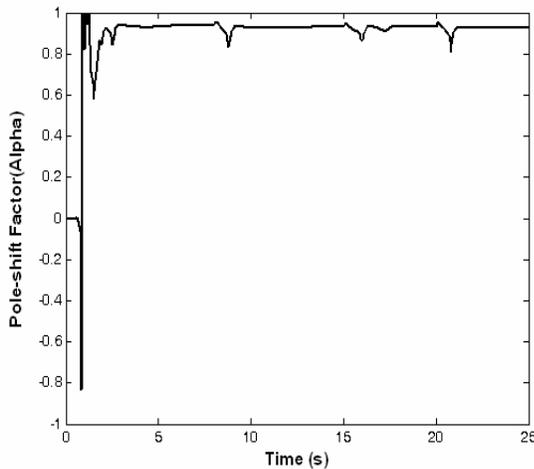
Fig. 5. The variation of the pole-shift factor with the progression of the adaptive process
