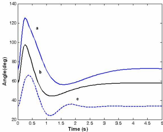
Fig. 10. Generator rotor angle variations following a three-phase fault for 0.1s with the proposed pole-shift control. The loadings are: a) 1.2 pu, b) 0.9 pu, and c) 0.5 pu.
