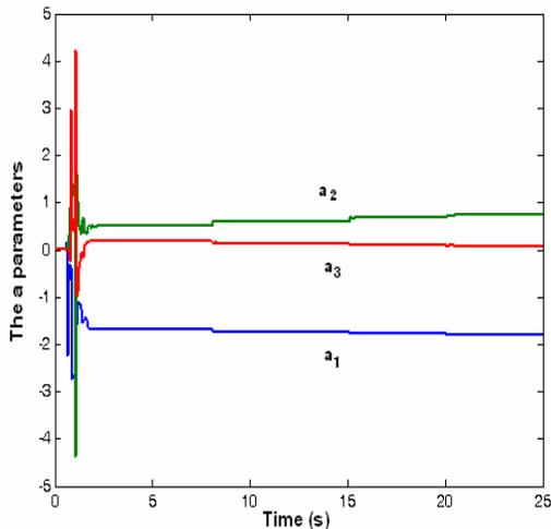
Fig. 6. The variation of the a-parameters of the adaptively identified plant function
