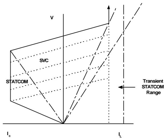
Fig. 3 V-I characteristic of STATCOM and SVC
