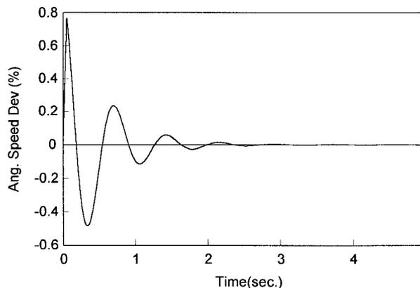
Fig.8 Generator speed variation of with robust controller in the speed loop.
