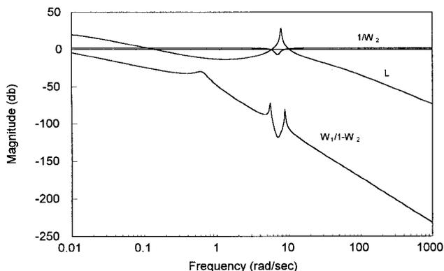
Fig. 6 Loop shaping plots relating  $W_1$ ,  $W_2$  and  $L$ .
