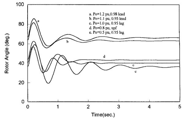
Fig.11 Generator power angle for various loading conditions
