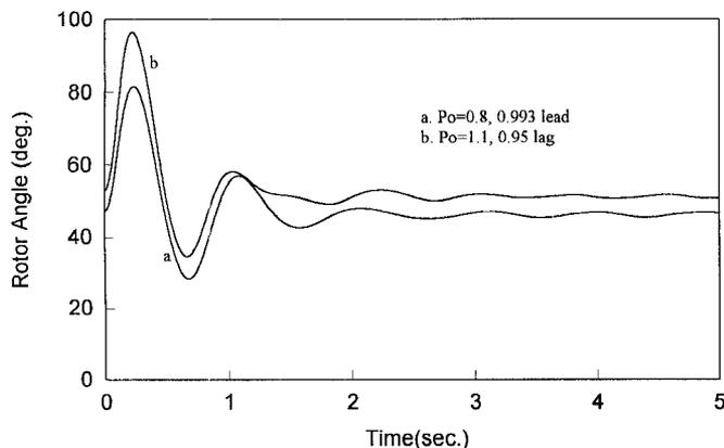
Fig.13 Generator angle variations following fault for 2 different operating conditions.
