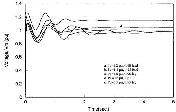
Fig.12. Bus voltage variations for various loading conditions.
