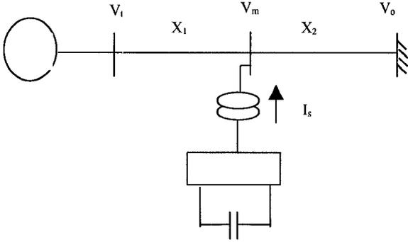
Fig.1 Single Machine System with STATCOM
