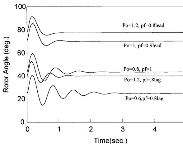
Fig.9 Load angle with the robust controller for various conditions.
