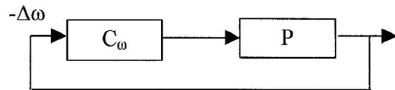
Fig 4 Collapsed block diagram for robust speed feedback system.
