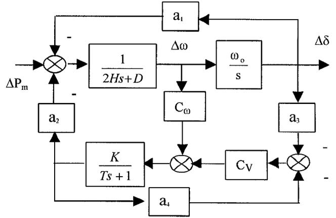
Fig.2 Block diagram of the linearized system.
