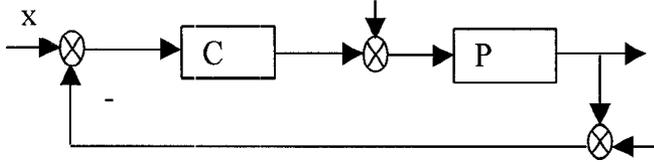
Fig.3 Unity feedback plant with controller.
