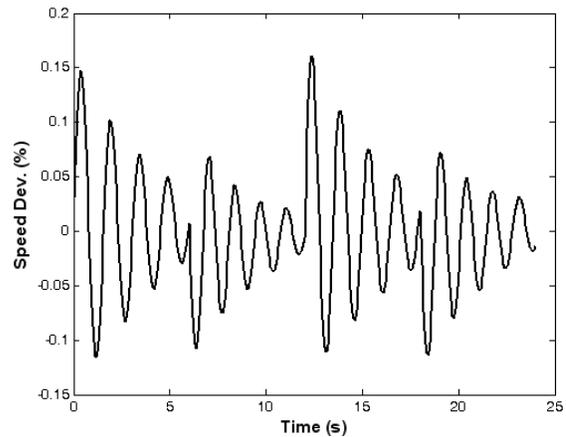
Figure 3 Generator speed variation with no control
