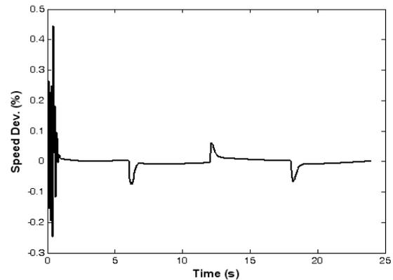
Figure 4 Generator speed deviation with the online adaptive stabilizing control
