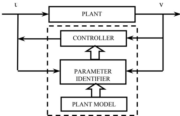
Figure 2 Block diagram of self-tuning controller
