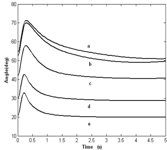
Fig. 11 Generator rotor angle variations following 50% torque pulse for 5 loading conditions.
