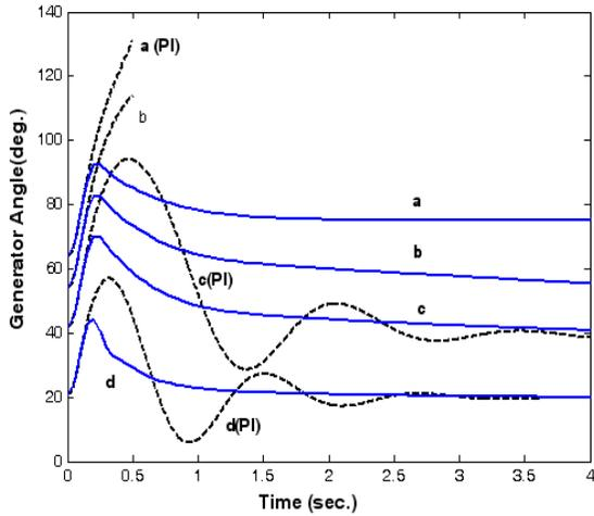
Fig. 9 Generator rotor angle characteristics following a 100% torque pulse of 0.1s for the 4 operating conditions with pole shift adaptive control (solid lines) and with PI controls (dotted lines).
