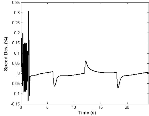
Figure 10 Generator speed variation corresponding to Fig.3 with adaptive pole-shift control
