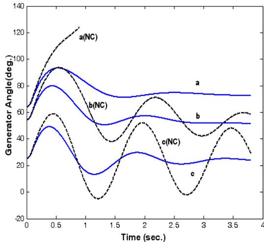
Fig.12 Generator rotor angle variations for a 50% torque pulse disturbance of 0.1s for three different operating conditions a, b and c with and without (NC) PI control.
