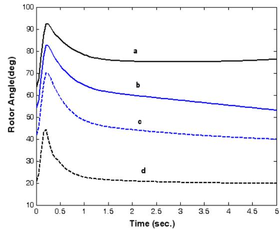
Figure 8 Generator rotor angle variations following 100% torque pulse for 5 loading conditions.
