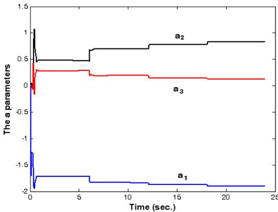
Figure 6 Online adaptations of the 'a' parameters in the model function
