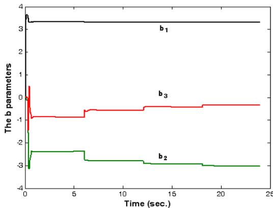
Figure 7 Online adaptations of the 'b' parameters
