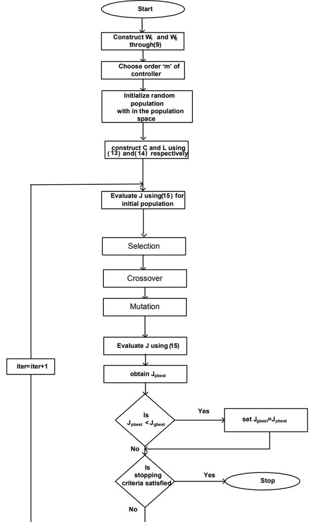
Fig. 2. Flow chart for the proposed automatic loop-shaping.
