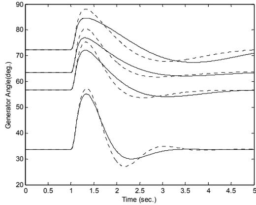
Fig. 7. Comparison of generator rotor angle variations following a 50% input torque pulse (solid line is for automatic loop-shaping and dotted line for graphical method).
