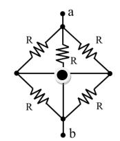
**b**) What is the equivalent resistance in term of *R* between points a-b?
