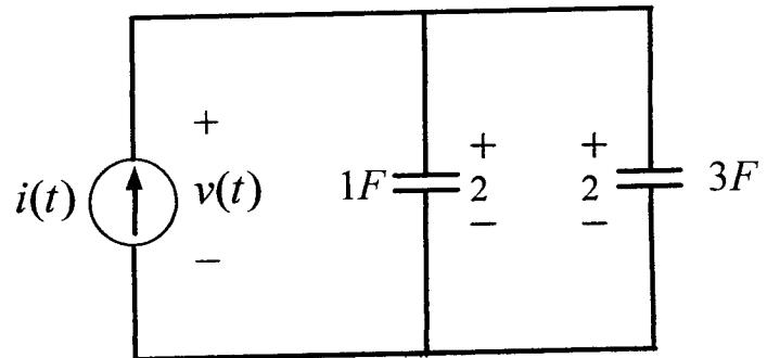
For the circuit shown above, the capacitors initially have 2 V.
