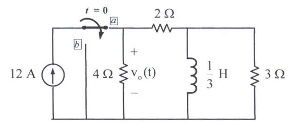
For the circuit shown above, the switch was in position a for a long time Find  $V_o(t)$  for all time ?
