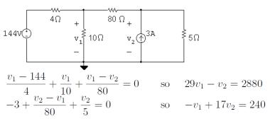
Solving,  $v_1 = 100 \text{ V}; \quad v_2 = 20 \text{ V}$
